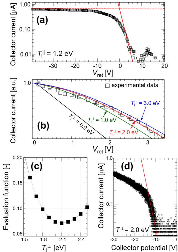
Fig. 2 (a)  $I$ - $V$  curve obtained with the RFA, (b) comparison with calculations, (c)  $f_{\text{er}}$  defined in Eq. (2) as a function of  $T_i^{\perp}$ , and (d)  $I$ - $V$  curve obtained with the ISP.
