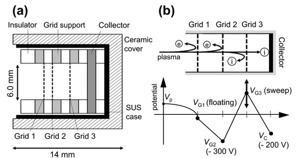
Fig. 1 (a) Cross-section of the RFA, and (b) potential structure within the RFA.
