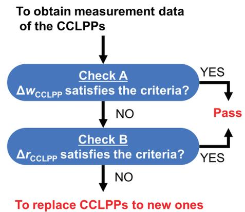
Fig. 3 Flow chart of the double check process.
