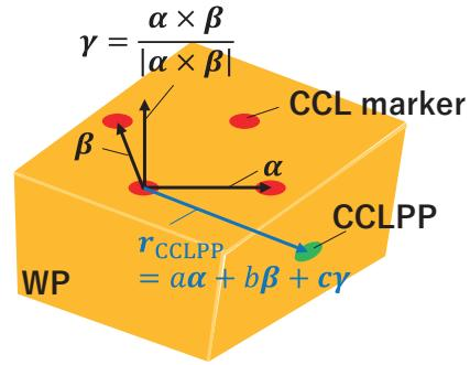
Fig. 4 Calculation of  $r_{\text{CCLPP}}$  in check B.
