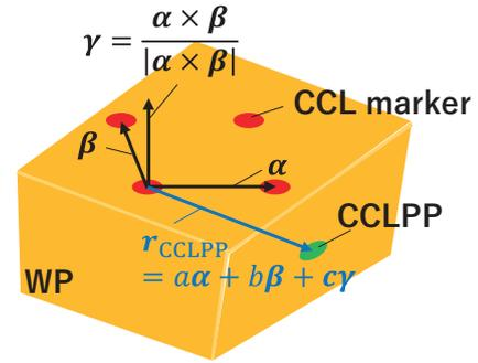
Fig. 4 Calculation of  $r_{\text{CCLPP}}$  in check B.
