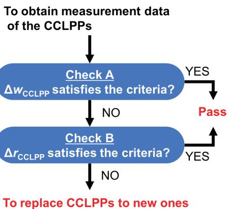
Fig. 3 Flow chart of the double check process.
