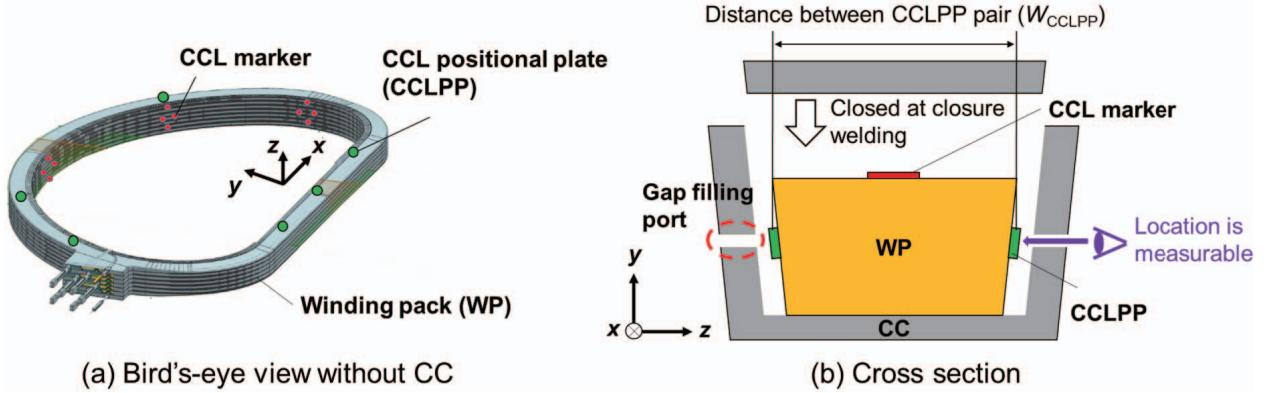
Fig. 1 The WP, CC, and markers used for the ITER TF coil integration.
