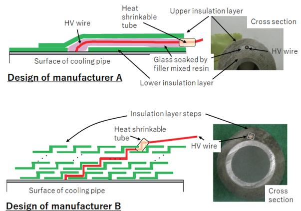
Fig. 14 Sketch of the design of HV wire exit by each manufacturer.
