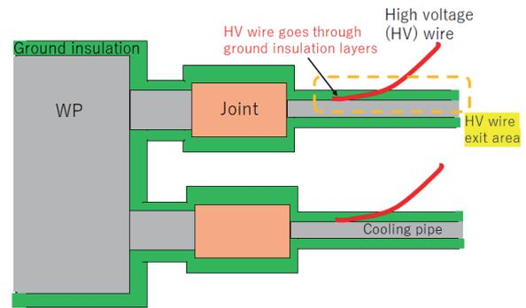
Fig. 13 Sketch of the HV wire installed on a WP.
