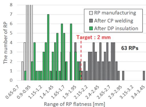
Fig. 10 Results of the DP flatness after DP insulation for all 63 DPs manufactured. Vertical and horizontal axes are the number of DPs and range of DP flatness, respectively.
