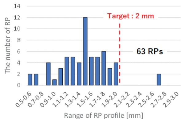
Fig. 5 Results of the RP profile for all 63 RPs manufactured. Vertical and horizontal axes display the number of RPs and range of RP profile, respectively.
