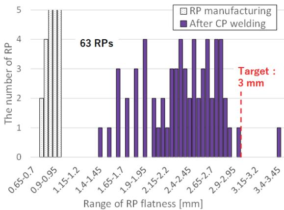
Fig. 7 Results of the RP flatness after CP welding for all 63 RPs manufactured. Vertical and horizontal axes display the number of RPs and range of RP flatness, respectively.
