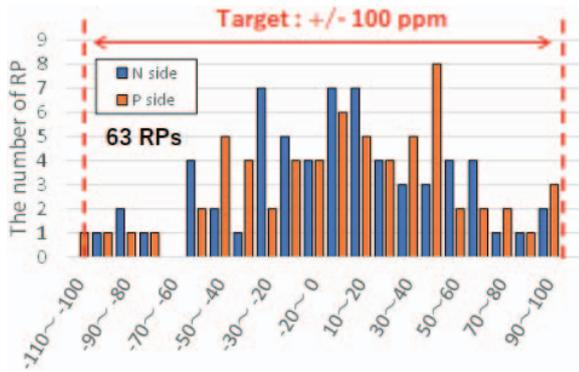
Fig. 6 Results of the RP groove-length variation for all 63 RPs manufactured. Vertical and horizontal axes display the number of RPs and range of groove-length variation, respectively.
