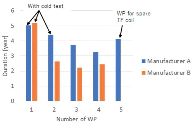
Fig. 17 WP manufacturing duration of each TF coil manufacturer.
