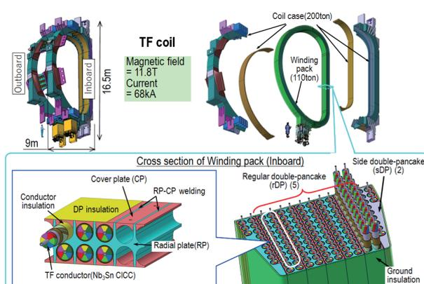
Fig. 1 Overview of an ITER TF coil.
