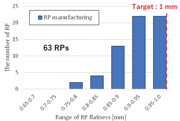
Fig. 4 Results of the RP flatness for all 63 RPs manufactured. Vertical and horizontal axes display the number of RPs and the range of RP flatness, respectively.
