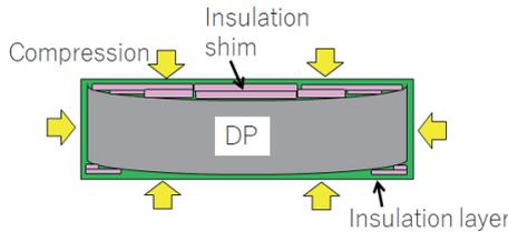
Fig. 9 Sketch of the DP insulation.
