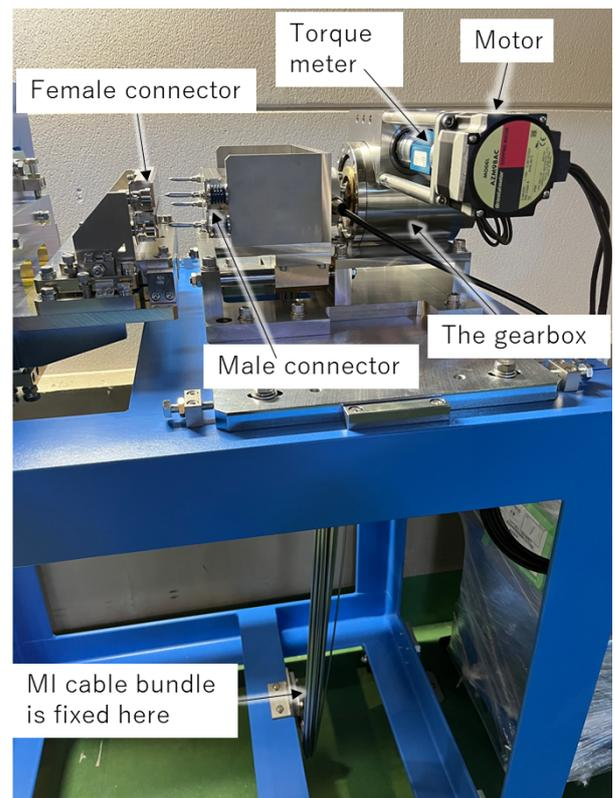
Fig. 4 The RHEC prototyping.
