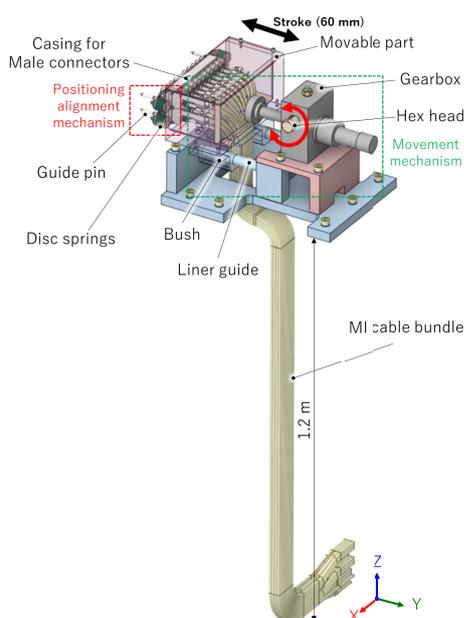
Fig. 2 Configuration of RHEC.
