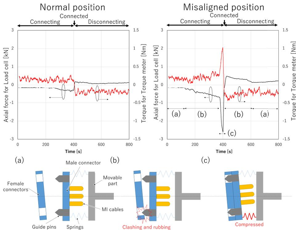
Fig. 6 The results of the axial force for the load cell and the torque for the torque meter, and pictures for each state; (a) connecting/disconnecting state, (b) touching/detaching state of the guide pins on the holes, and (c) Connected state.
