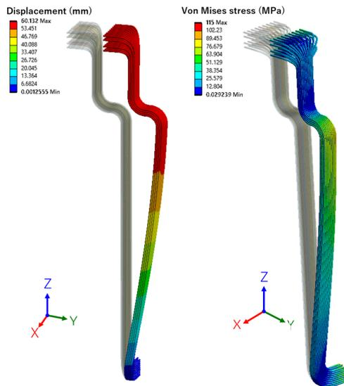
Fig. 3 Analysis result Displacement (left) and Von Mises stress (Right) showing the original position as the shadow.
