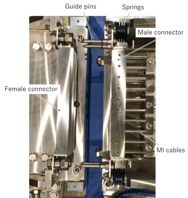
Fig. 5 The magnification picture of the connectors.
