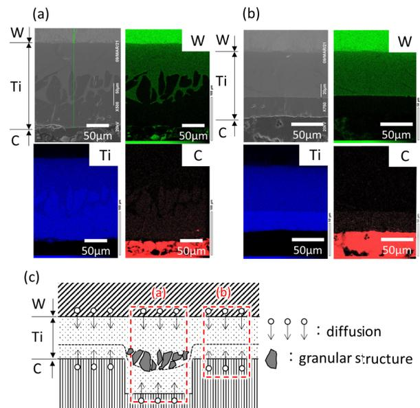
Fig. 4 SEM images and composition mapping images in (a) the grooved area, and (b) non-grooved area, (c) Schematic view of the bonding interlayer.
