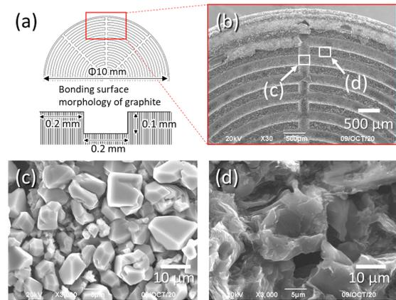
Fig. 3 The fracture surface of a bonding specimen with groove on graphite. (a) Groove pattern, (b) SEM image of the fracture surface, (c) SEM image of grooved area, and (d) SEM image of non-grooved area. There is granular structure in the grooved area.
