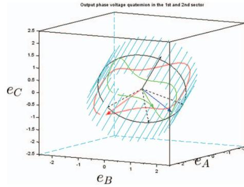
Fig. 3 Output phase voltage quaternion in the direct matrix converter. The output line voltage quaternion (a circle) is also displayed.
