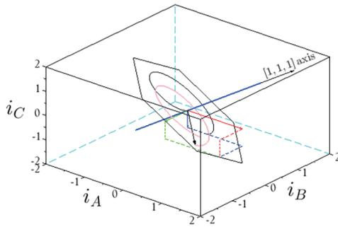
Fig. 5 Output phase current quaternion in a transition phase to switching configuration (+1) or (1, 2, 2). Blue line: zero-sequence current quaternion; red line: positive-sequence current quaternion; black curve: negative-sequence current quaternion.
