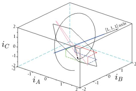
Fig. 6 Output phase current quaternion in a transition phase to switching configuration (+1) or (1, 2, 2). Blue line: zero-sequence current quaternion; red line: positive- and negative-sequence current quaternion; black curve: the sum of zero-, positive-, and negative-sequence current quaternion.
