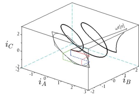
Fig. 4 Time evolution of three-phase AC output phase current quaternion in matrix converter.
