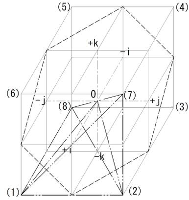
Fig. 1 Quaternion of three-phase AC phase voltage in a voltage-source inverter.
