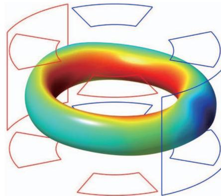
Fig. 1 Arrangement of saddle coils and the  $|B|$  distribution on the last closed flux surface. The colors of saddle coils indicate the direction of current.
