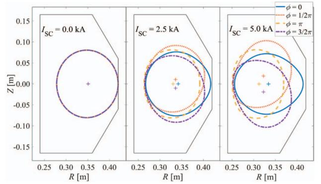
Fig. 2 LCFS with  $I_{SC} = 0.0$  kA (left),  $I_{SC} = 2.5$  kA (middle),  $I_{SC} = 5.0$  kA (right). Makers of ‘‘+’’ and black hexagon indicate the positions of magnetic axes and the limiter of PHiX, respectively.
