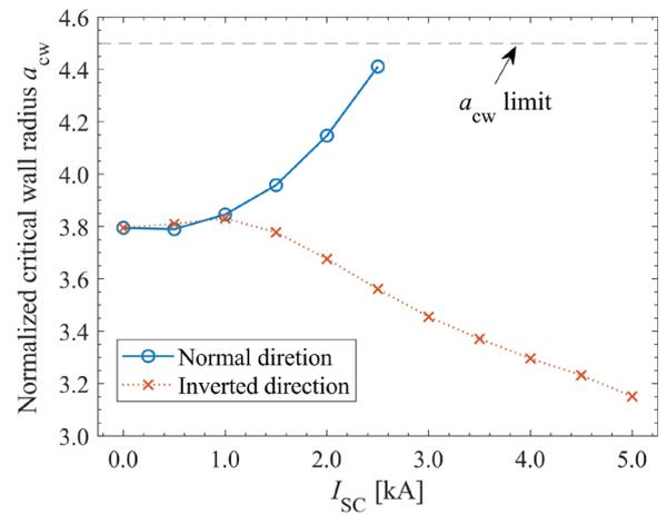
Fig. 6 Normalized critical wall radius  $a_{cw}$  versus  $I_{SC}$ . Makers of “o” and “x” indicate a  $a_{cw}$  of the saddle coils current in normal direction and inverted direction, respectively.
