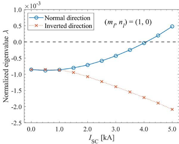
Fig. 4 Normalized eigenvalue versus  $I_{SC}$ . Makers of “o” and “x” indicate  $\lambda$  of the saddle coils current in normal direction and inverted direction, respectively.
