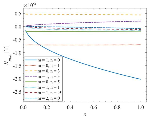
Fig. 3 Boozer spectrum of the equilibrium with  $I_{SC} = 5.0$  kA. The Fourier mode of  $B_{00}$  is excluded.
