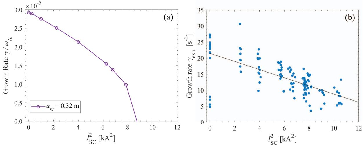
Fig. 7 Comparison between the growth rate calculated by TERPSICHORE (a) and the growth rate obtained experimentally (b). The line in Fig. 7 (b) is the result of a linear fitting.
