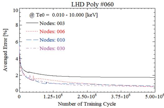
Fig. 3 Averaged error as a function of the number of nodes ( $N_{tr}$ ) for  $N_{nodes} = 3, 6, 10,$  and  $30$ .
