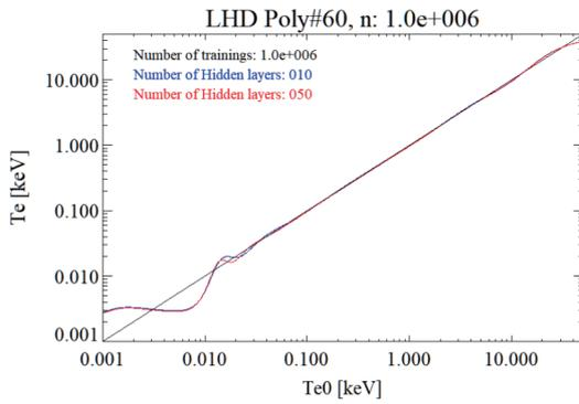
Fig. 4 Comparison between target temperature  $T_e^0$  and final result  $T_e$  after completing the training course for  $N_{node} = 10$  (blue) and  $50$  (red).
