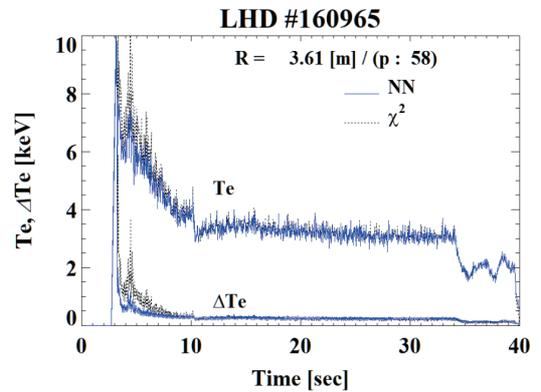
Fig. 5 (b) Comparison of time histories of  $T_e$  at the plasma center obtained by the NN and minimum  $\chi^2$  methods.
