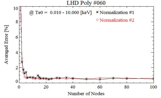
Fig. 2 Averaged error as a function of the number of nodes ( $N_{\text{nodes}}$ ). The errors are estimated in the  $T_e$  range,  $T_e = 10 \text{ eV} - 10 \text{ keV}$ .
