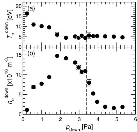
Fig. 3 (a) Electron temperature, and (b) electron density obtained at the secondary gas feeding position as a function of downstream pressure.
