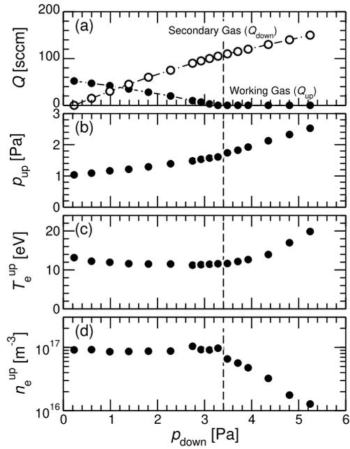
Fig. 2 (a) The amount of working and secondary gases, (b) neutral pressure, (c) electron temperature, and (d) electron density as a function of downstream pressure. Values shown in panels (b), (c), and (d) were obtained near the plasma production region.
