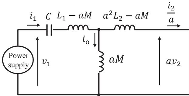
Fig. 3 An equivalent circuit converted to the primary side of an air-core HTS transformer connected with a resonant capacitor.
