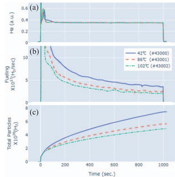
Fig. 16 Particle fueling at different CS temperatures. (a)  $H\alpha$  emission controlled to 0.35 (a.u.), (b) fueling rate by MFC, (c) total fueled particle.
