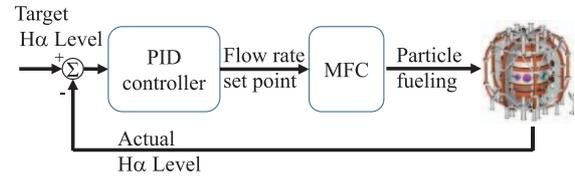
Fig. 4 Particle fueling feed-back control with  $H\alpha$  signal.
