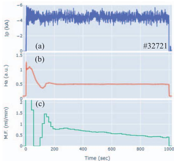
Fig. 6 Test result of feedback control of  $H\alpha$  emission intensity by MFC. (a) Plasma current, (b)  $H\alpha$  emission intensity, and (c) fueling rate by MFC.
