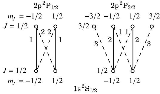
Fig. 1 Kastler diagram for the Lyman- $\alpha$  line. The solid and dashed lines correspond to the  $\Delta m_J = 0$  and  $\Delta m_J = \pm 1$  transitions, respectively. The numbers next to the lines indicate the relative line intensities when the population in the upper state is equally distributed over all the magnetic sublevels.
