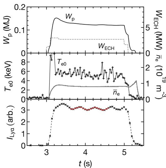
Fig. 6 Example of discharge for the measurement: (a) ECH power and stored energy, (b) line-averaged electron density and central electron temperature, and (c) Lyman- $\alpha$  line intensity of the present observation.
