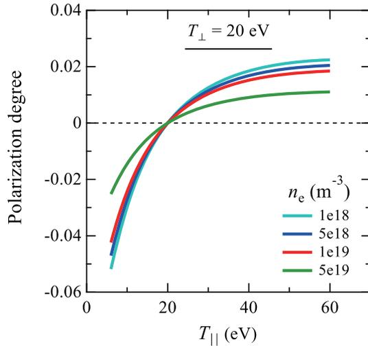
Fig. 3 Simulation results for the polarization degree as a function of  $T_{\parallel}$  under a fixed  $T_{\perp}$  at 20 eV. The influence of the unpolarized line  $1^2S_{1/2} - 2^2P_{1/2}$  is included.
