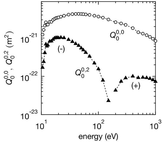
Fig. 2 Cross sections for the excitation  $Q_0^{0,0}$  [6] and alignment creation  $Q_0^{0,2}$  [7] for calculating their rate coefficients  $C^{0,0}(1, p)$  and  $C^{0,2}(1, p)$ , where  $p$  stands for the state  $2^2P_{3/2}$ . The label (-) indicates that true values take negative sign.
