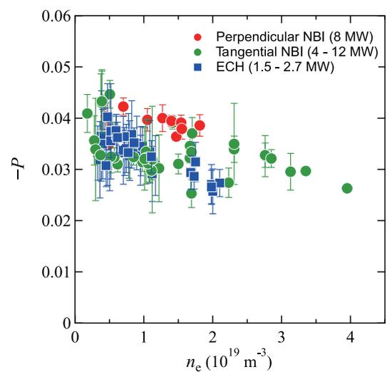
Fig. 7 Measurement results of the polarization degree plotted against  $\bar{n}_e$  for some different heating conditions. The red and green circles show results with the perpendicular NBI and tangential NBI, respectively, and the blue squares show results with the ECH.
