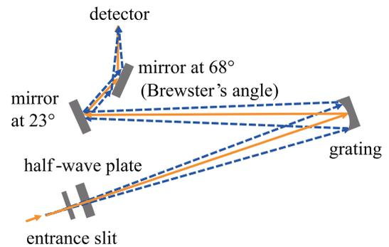
Fig. 5 Schematic drawing of the spectrometer. Two mirrors and a half-wave plate are supplementary installed for the polarization measurement.
