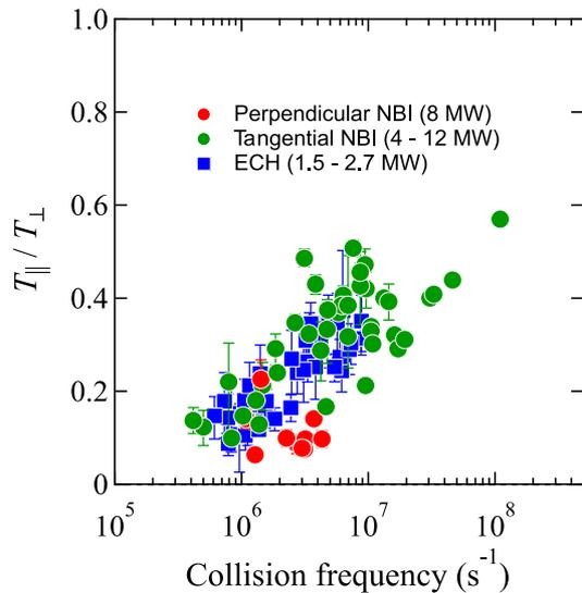
Fig. 8 Anisotropy in terms of  $T_{\parallel}/T_{\perp}$  plotted against the electron-electron collision frequency at the expected emission location  $r_{\text{eff}} = 0.67$  m.
