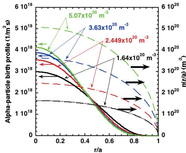
Fig. 9 The birth profile of fusion-born alpha particles and corresponding densities with the same profile  $\alpha_n = 0.5$ .
