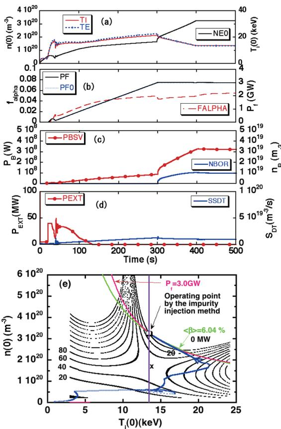
Fig. 1 Temporal evolution of the plasma parameters in FFHR-d1 operated in the stable ignition regime with impurity injection ( $\alpha_n = 0.5$ , and the confinement factor  $\gamma_{04} = 1.3$  over ISS04 scaling). (a) Ion temperature and electron temperature and the density, (b) Fusion power and the alpha ash fraction, (c) the bremsstrahlung radiation and impurity density and (d) external heating power and fueling rate, (e) The operating path on the POPCON.
