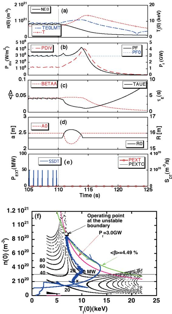
Fig. 6 Temporal evolution of the plasma parameters after stopping fueling with the plasma shift model during the unstable operation. (a) - (f) are the same as in Fig. 4.
