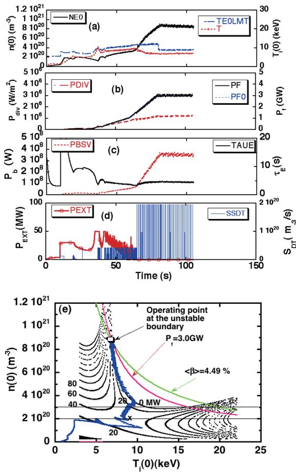
Fig. 3 Temporal evolution of the plasma parameters directly accessed to the unstable ignition regime by fueling ( $\alpha_n = 3.0$  and the confinement factor  $\gamma_{95} = 1.43$  over ISS95 scaling). (a) - (e) are the same as in Fig. 1 except for (c) the bremsstrahlung radiation and confinement time.
