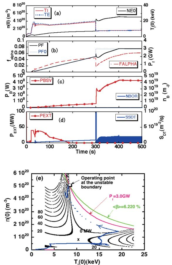
Fig. 2 Temporal evolution of the plasma parameters in FFHR-d1 operated in the unstable ignition regime by fueling through the stable operation regime just for comparison with impurity injection ( $\alpha_n = 0.5$  and the confinement factor  $\gamma_{04} = 1.3$ ). (a) - (e) are the same as in Fig. 1.
