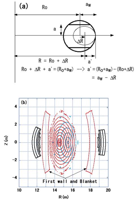
Fig. 5 (a) The limiter model to simulate the plasma shift effect, and (b) the magnetic surface behavior when the plasma shifts outward (from red to blue contours).
