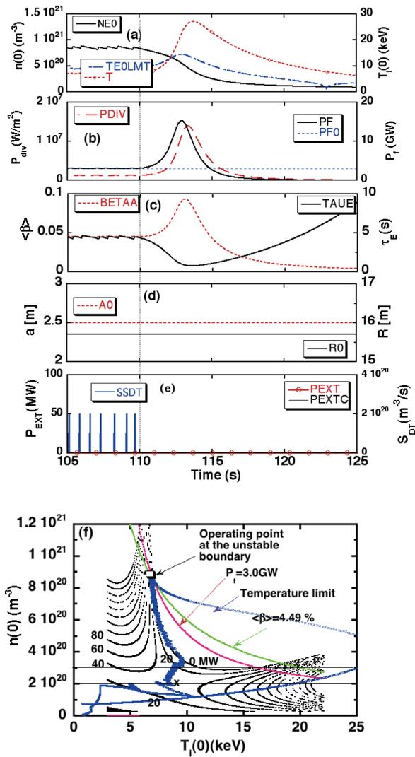
Fig. 4 Temporal evolution of the plasma parameters after stopping fueling during the unstable operation ( $\alpha_n = 3.0$  and the confinement factor  $\gamma_{95} = 1.43$ ). (a) The temperature and the density, (b) fusion power and divertor heat load, (c) the beta and confinement time, (d) plasma position, (e) external heating power and fueling rate, and (f) the operating path on the POPCON.
