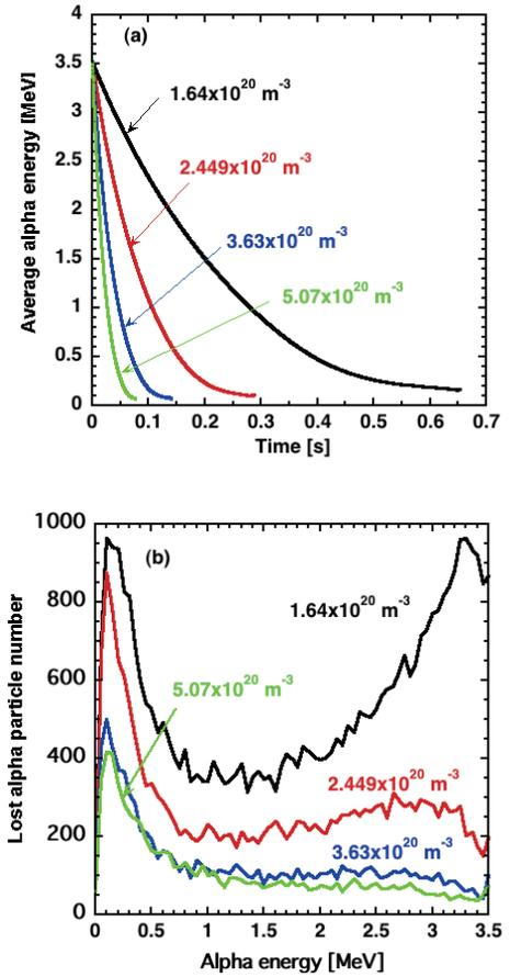
Fig. 8 (a) Time dependence of the average alpha energy, and (b) the lost alpha particle counting number vs. the alpha energy for various ignition densities with  $\alpha_n = 0.5$ .
