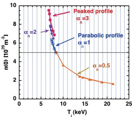
Fig. 7 Dependence of the operating density on the temperature for ignited operation for various profile parameters  $\alpha_n$ .
