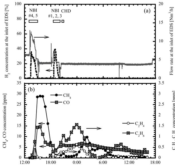
Fig. 5 Variations of the gas species in the exhaust gas during the regeneration operation of the cryosorption pump for the NBI and CHD: (a) Concentrations of hydrogen and the exhaust gas flow, and (b) concentrations of the hydrocarbons and carbon monoxide.
