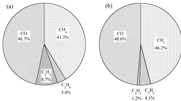
Fig. 6 The ratio of gas species in the exhaust gas: (a) Glow discharge cleaning operation, and (b) regeneration operation of cryosorption pumps for the NBI and CHD.
