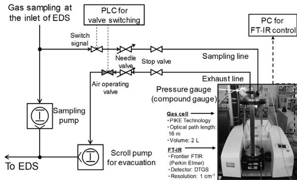
Fig. 1 Schematic diagram of the FT-IR system.
