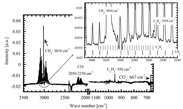
Fig. 2 An example FT-IR spectrum obtained during the  $\text{H}_2$  glow discharge cleaning operation in the LHD. The vertical bars in the sub graph represent the absorption lines of  $\text{C}_2\text{H}_6$  and  $\text{CH}_4$ .
