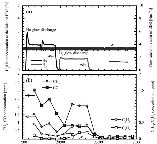
Fig. 4 Variations of the gas species in the exhaust gas during the helium and H<sub>2</sub> glow discharge cleaning operations: (a) Concentrations of hydrogen, helium and the exhaust gas flow, and (b) concentrations of the hydrocarbons and carbon monoxide.
