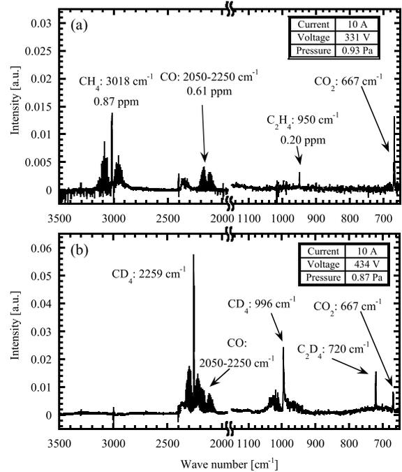
Fig. 7 FT-IR spectrum of the exhaust gas during the glow discharge cleaning operation. The conditions of glow discharge cleaning are shown in each graph. (a) H<sub>2</sub> glow discharge, and (b) D<sub>2</sub> glow discharge.
