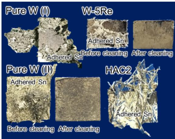
Fig. 1 Results of visual inspection on specimens after corrosion tests.
