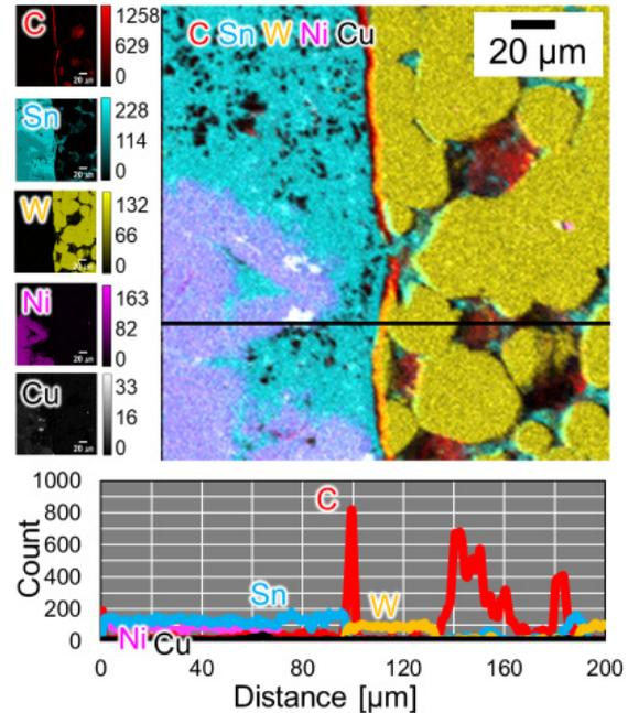
Fig. 3 Results of surface cross-sectional EPMA analysis on HAC2 specimen.
