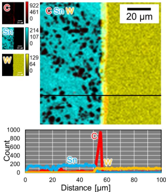
Fig. 2 Results of surface cross-sectional EPMA analysis on pure W (I) specimen.
