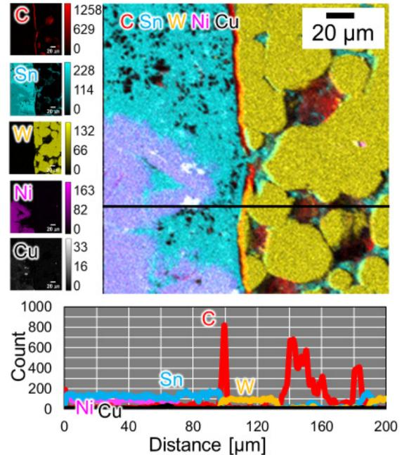
Fig. 3 Results of surface cross-sectional EPMA analysis on HAC2 specimen.
