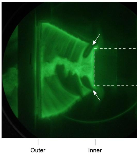
Fig. 3 Gated image of the z pinch of divergently aligned two wires. The white dotted line shows the inner electrode. The wires were interrupted at the positions shown by arrows.
