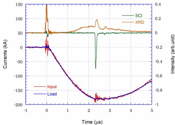
Fig. 2 Discharge currents and radiation signals (SCI and XRD) of the z-pinch discharge.
