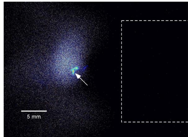
Fig. 4 Soft x-ray pinhole image of the z-pinch plasma. The white dotted line shows the inner electrode. A hot spot was generated in front of the inner electrode.
