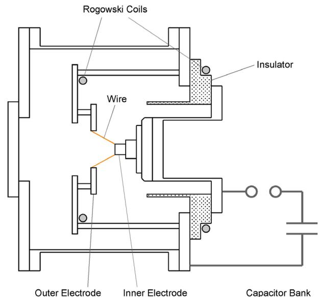
Fig. 1 Experimental set up of the z pinch of divergently aligned two wires on the SHOTGUN III-U device.
