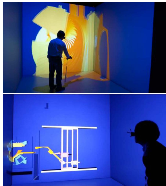
Fig. 15 Application of Virtual-Reality (VR) to the fusion engineering. The viewer grasps the component by his virtual hand (top). The viewer watches the movement of component by the robot system (bottom).
