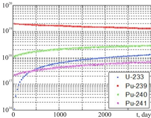
Fig. 6 Nuclear density of various isotopes in radioactive waste component in the fuel, nucl/cm<sup>3</sup>.
