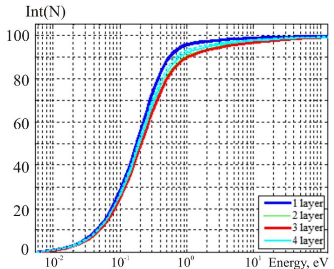
Fig. 5 Percentage of neutrons with energy less than one pointed on the axis (at the beginning of operation).
