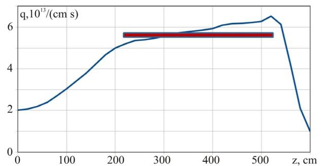
Fig. 2 Distribution of neutron emission from plasma column in the region of the subcritical assembly (the region is marked by a brown bar).
