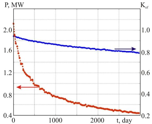
Fig. 4 Effective multiplicity coefficient ( $k_{ef}$ , blue curve) and power of subcritical assembly ( $P$ , red curve) vs. operation time.
