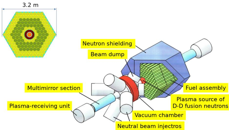
Fig. 1 Schematic of facility for studying the evolution of thorium-plutonium fuel composition.
