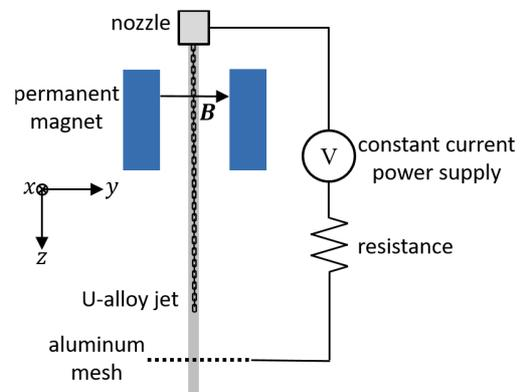
Fig. 2 Schematics of the experimental setup. The origin of the Cartesian coordinate is set just below the nozzle.
