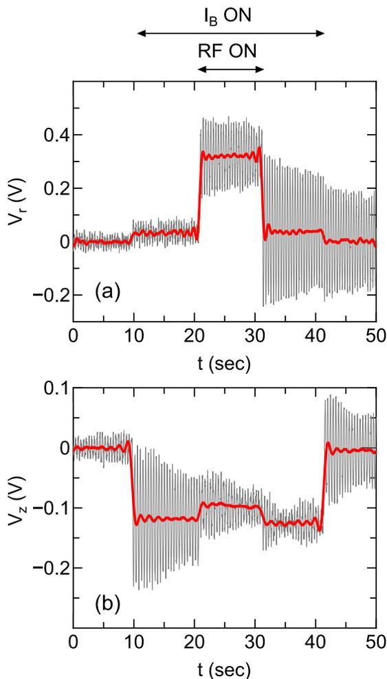
Fig. 4 The LED displacement sensor signals in the (a) radial and (b) axial directions, where the solenoid current  $I_B$  and the rf power are turned on for  $t \sim 10 - 40$  sec and for  $t \sim 20 - 30$  sec, respectively. The positive changes of the signals indicate that the radially outward and axially downstream forces are exerted to the detector plate.
