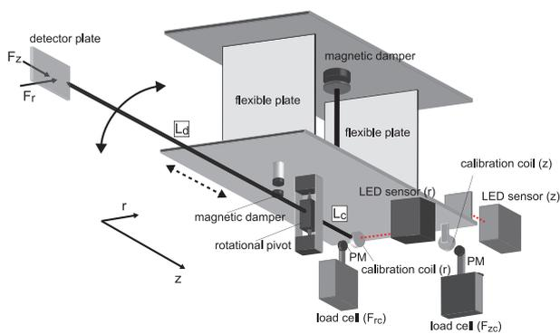
Fig. 1 Schematic diagram of the momentum vector measurement instrument (MVMI), where the whole structure is flipped from the previous bench test [22].
