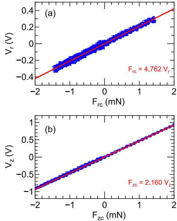
Fig. 3 The measured forces and the displacement sensor signals (dots) when sweeping the currents of the (a) radial and (b) axial calibration coils. The bold solid lines show the fitted linear lines giving the calibration coefficients shown by the inset texts in Fig. 3.
