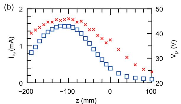
Fig. 2 (a) Schematic diagram of the experimental setup. (b) Measured ion saturation current  $I_{is}$  (open squares) and the local plasma potential  $V_p$  (crosses) on axis.
