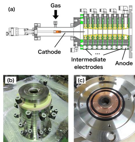
Fig. 1 Developed PW: (a) schematic of the PW; (b) overall view of the PW; (c) internal structure of the intermediate electrode.
