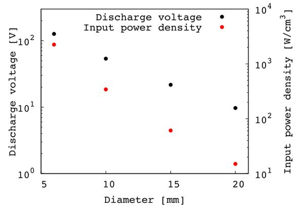
Fig. 4 Discharge voltage and average input power density as a function of diameter.
