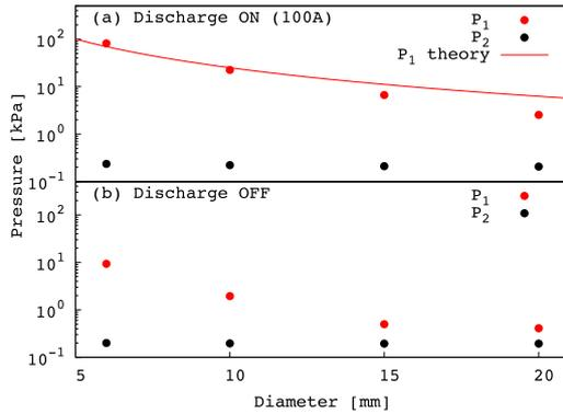
Fig. 3 Measured  $P_1$ ,  $P_2$ , and theoretical  $P_1$  as a function of diameter.
