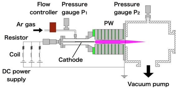
Fig. 2 Experimental setup.
