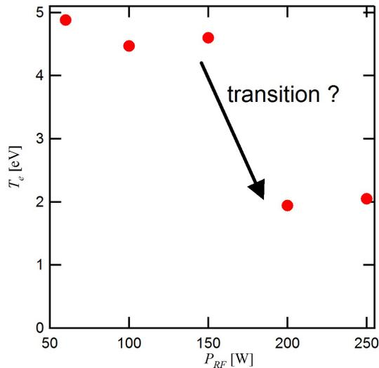
Fig. 4 Dependence of  $T_e$  on  $P_{RF}$  in the source, indicating that  $T_e$  can increase to approximately 5 eV with a  $P_{RF}$  that is below 150 W. In these experiments,  $n_e$  has been inferred to be  $\approx 4 \times 10^{15}$  and  $\approx 1 \times 10^{16} \text{ m}^{-3}$  for cases where  $P_{RF} = 100$  and 250 W, respectively, suggesting that the plasma pressure is kept almost constant as long as  $P_{RF}$  is varied below 250 W.
