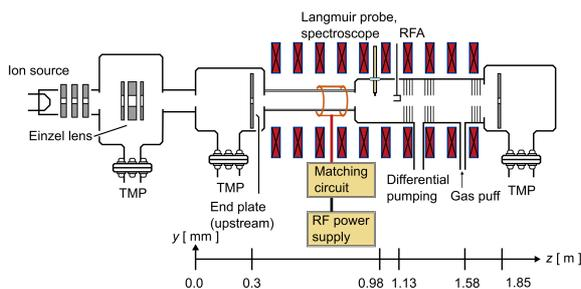
Fig. 1 Schematic of the DT-ALPHA device.
