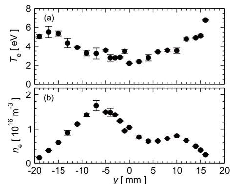
Fig. 2 Radial profile of the (a) electron temperature and (b) electron density obtained at  $z = 0.98$  m.
