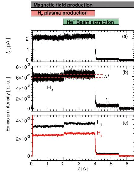
Fig. 3 Time evolution of the (a) collector current, (b)  $H_\alpha$  emission intensity, and (c)  $H_\beta$  and  $H_\gamma$  emission intensities.
