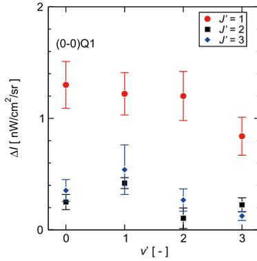
Fig. 5 Increase in the emission intensity of the Fulcher- $\alpha$  band owing to ion collision as a function of the vibrational quantum number of the upper excited state.
