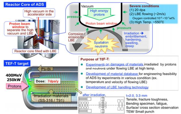
Fig. 5 The proton beam window of ADS under severe circumstances and purposes of TEF-T.
