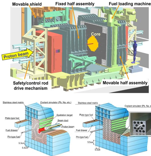
Fig. 4 Schematic view of the critical assembly to be installed in TEF-P.
