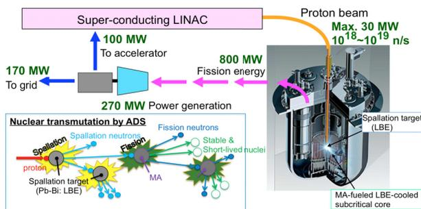
Fig. 1 A typical example of ADS.
