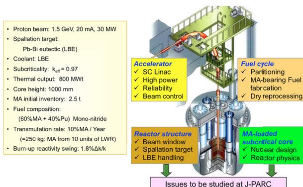
Fig. 2 A commercial ADS design proposed by JAEA with major parameters.
