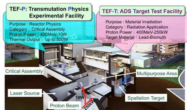
Fig. 3 Conceptual drawing of J-PARC Transmutation Experimental Facility (TEF).
