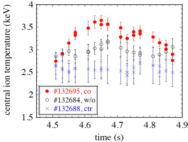
Fig. 4 Time evolutions of central ion temperature in the co-ECCD, counter-ECCD, and no ECCD discharges. The results were obtained by temporal averaging of each set of three neighboring data points in the original data.
