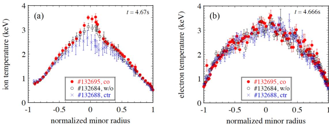
Fig. 3 (a): Radial profiles of ion temperature diagnosed by CXS measurements at  $t = 4.67$  s in the co-ECCD, counter-ECCD, and no ECCD discharges. The results were obtained by spatial averaging of each set of three neighboring data points in the original data. (b): Radial profiles of electron temperature diagnosed by Thomson scattering measurements at  $t = 4.666$  s.
