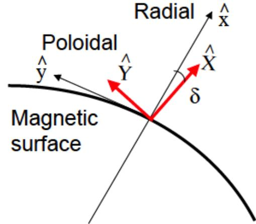
Fig. 19 Possible mis-alignment of Reynolds stress probe. The Cartesian coordinates on the probe array ( $X, Y$ ) are inclined by the small angle  $\delta$ , with respect to the radial-poloidal coordinates ( $x, y$ ) on magnetic surface.
