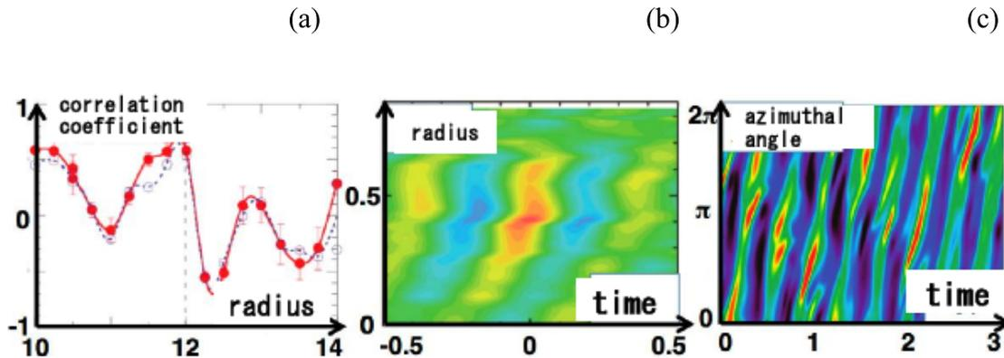
Fig. 1 Experimental confirmations of meso- and macroscopic perturbations in toroidal plasmas. Spatiotemporal correlations of zonal flow (a), global fluctuation (b) and streamer (c), respectively. Based on [46,48,50].
