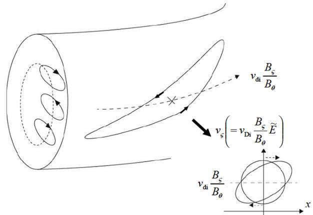
Fig. 7 Conversion of toroidal flow from poloidal flow. The precession of trapped particles is modified by the fluctuating electric field. A vortex in the phase space is inclined, so that the net toroidal torque remains [87]. This is compared with the conventional understanding of Reynolds stress, which is generated by the vortex in the real space.
