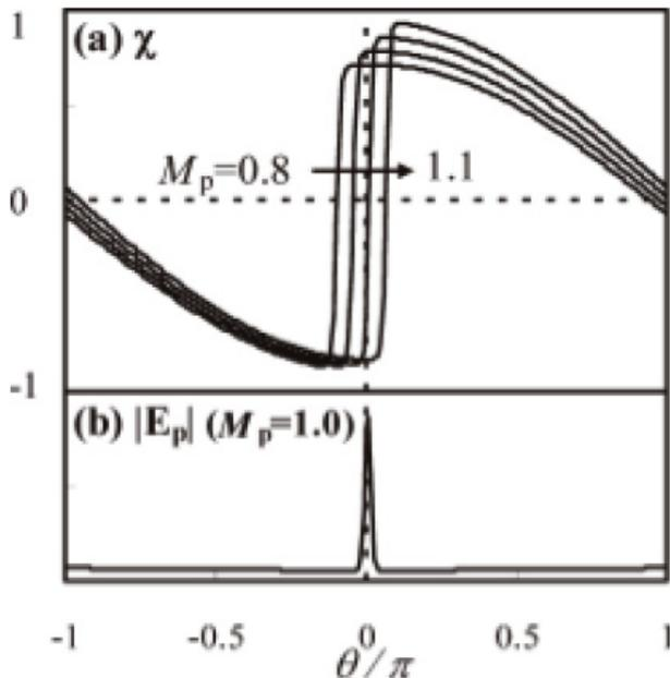
Fig. 6 Poloidal profile of normalized perturbed density (shown by natural log) (a) and magnitude of poloidal electric field for the case of  $M_p = 1$  (b), in the presence of strong radial electric field near plasma surface. The poloidal Mach number is close to unity. The poloidal shock is formed near  $\theta \sim 0$  (low field side midplane) in the present case. (Quoted from [85].)
