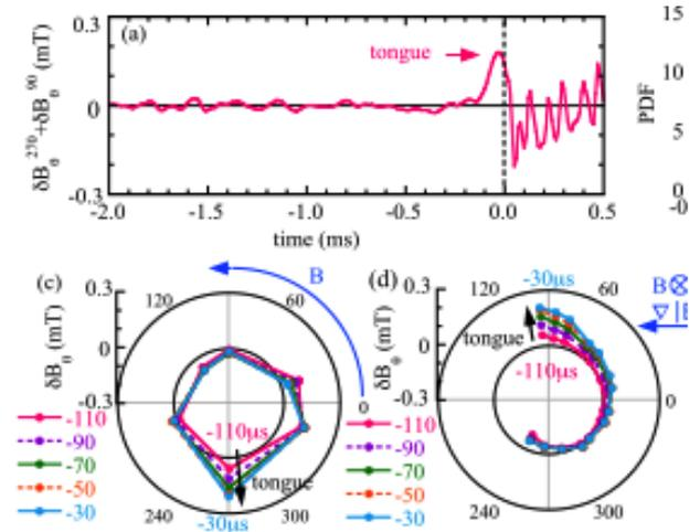
Fig. 9 ‘Tongue’ in abrupt burst which was observed on LHD [111]. Time evolution of sum of magnetic field  $B_\theta$  at  $\phi = 90$  and  $270^\circ$  in toroidal array. Polar plot of magnetic field perturbation  $B_\theta$  of (c) toroidal array and (d) poloidal array during the ‘tongue’ event ( $t = -110, -90, -70, -50$  and  $-30 \mu\text{sec}$ ).
