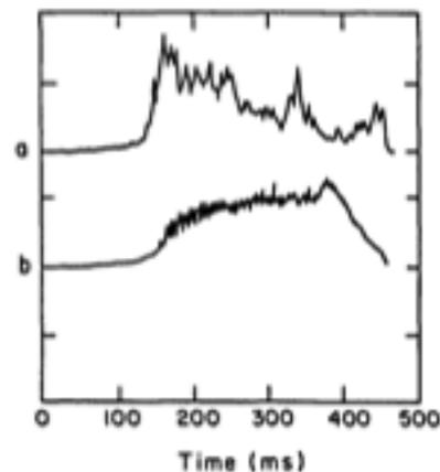
Fig. 16 Enhanced fluctuation at the onset of MARFE was observed on ALCATOR-C [80]. In this figure, line (a) indicates the line-averaged value of square of microscopic density fluctuation, which was measured by single-beam  $CO_2$  laser scattering. In this discharge the MARFE begins at 150 ms. It was reported that increase over two orders of magnitude in scattered power was observed when the scattering volume intersects the MARFE region. (Quoted from [114].)
