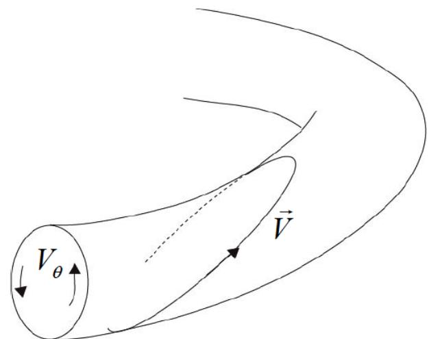
Fig. 5 Toroidal return flow is associate with the poloidal flow in the toroidal plasma [77].
