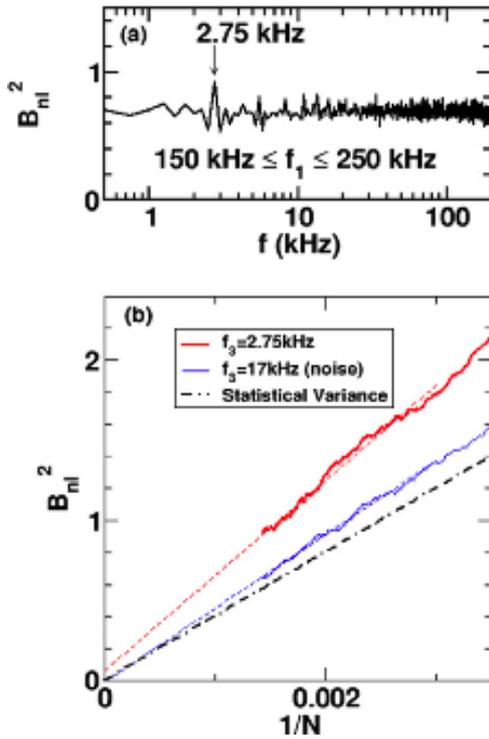
Fig. 18 An example of measurement of nonlinear interaction of microscopic turbulence at far distance. Quoted from [120]. Summed bi-coherence (which is a sum over the frequency range of  $150 \text{ kHz} < f_1 < 250 \text{ kHz}$ ). Signal at the frequency  $f_3$  is obtained at  $r/a = 0.63$ , while those at  $f_1$  and  $f_2$  are measured at  $r/a = 0.88$ . (b) Convergence study for the summed bi-coherence.
