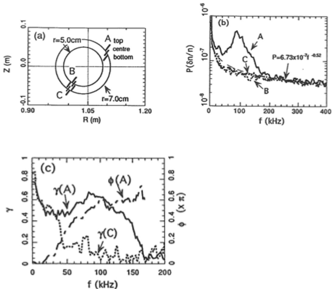
Fig. 3 Localization of turbulence intensity in the outside of torus. Measurements on the TEXT tokamak [73]. Poloidal asymmetry in density fluctuation spectra: (a) sample volume location, (b) power spectra, and (c) coherence between signals from two adjacent sample volumes and the phase difference on the low field side.
