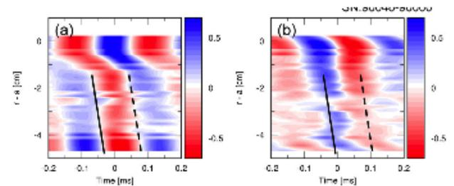
Fig. 10 Ballistic propagation of perturbation in turbulence amplitude near the edge of JFT-2M tokamak. Periodic modulation is induced by Limit Cycle Oscillation near plasma surface, and modulations of turbulence intensity and density gradient penetrate into the core plasma [79].
