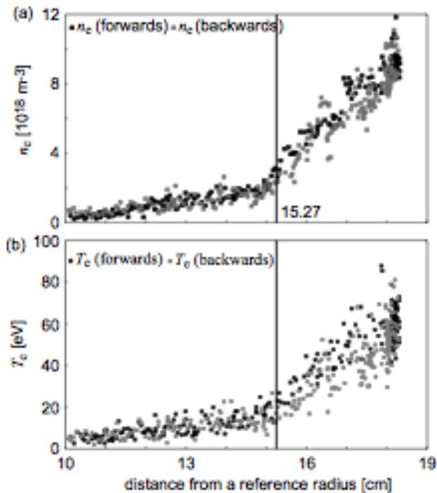
Fig. 22 Radial profiles of plasma parameters obtained by single Langmuir probe current-voltage Characteristic curves. (a) Electron density and (b) electron temperature, respectively. Plots during Forward and backward motions of the RLP are accompanied in both figures. Vertical lines indicate the position of plasma surface, which is estimated by cross points of the fitted asymptotic lines in the GAM amplitude profile. (Quoted from [124].)
