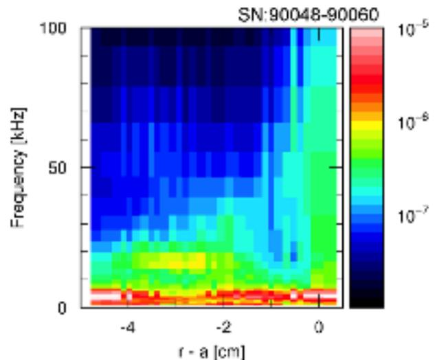
Fig. 17 Strong spatial inhomogeneity of turbulence near the plasma edge of the L-mode plasma in JFT-2M [119].
