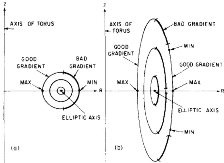
Fig. 2 Trapped particles and magnetic geometry. Shaping of magnetic surface can control distribution of trapped particles [72]. Effect of ellipticity on the instability. (a) circular tokamak and (b) elliptic tokamak. ‘max’ and ‘min’ denote the local extrema of B on the field line.
