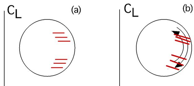
Fig. 8 Schematic illustration of dynamic shearing of ambient fluctuations by GAM. Contours of phases of toroidal fluctuations are shown by thick lines in (a). In the presence of poloidally-symmetric shearing motion, the phase contours are modified with up-down asymmetry. (Quoted from [82].)
