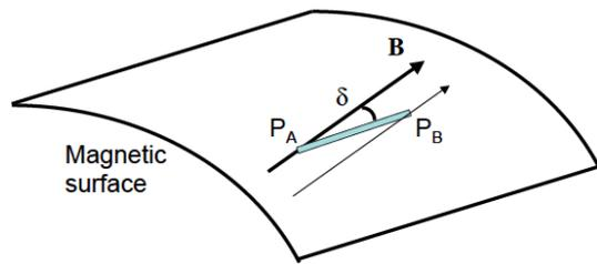
Fig. 20 Misalignment of the Mach probe. The probes at two ends of a Mach probe,  $P_A$  and  $P_B$ , are not on the same magnetic field line. Owing to the perpendicular wave number of fluctuations, the density fluctuation takes different values at  $P_A$  and  $P_B$ . This density difference is a source of error in the evaluation of the fluctuating Mach number.
