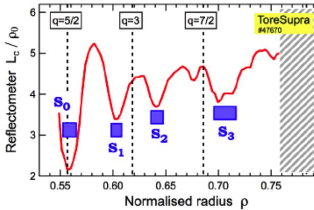
Fig. 11 Radial variation of the correlation length of fluctuations [103]. The reflectometer coherence length is plotted against radius (Tore Supra).
