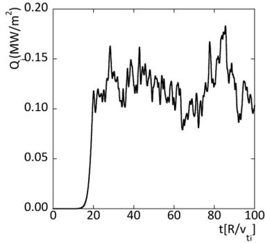
Fig. 1 Time evolution of the ion energy flux.
