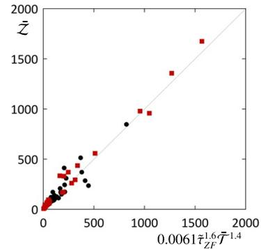
Fig. 4 The plots for the comparison of  $\bar{\mathcal{Z}}$  with  $0.0061 \bar{\tau}_{ZF}^{1.6} \bar{\mathcal{T}}^{1.4}$ . The circles show the simulation results in the high- $T_i$  phase and the boxes represent those in the low- $T_i$  phase.
