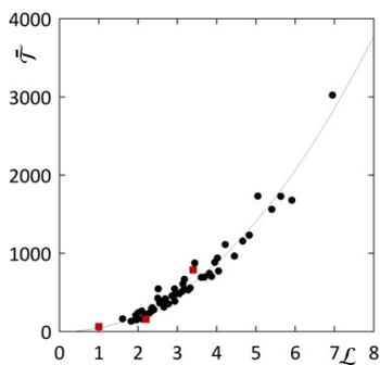
Fig. 3 Comparison of the time-averaged turbulent fluctuation  $\bar{\mathcal{T}}$  with the mixing length estimate,  $\mathcal{L}$ . The circles and the boxes represent the results in high- $T_i$  and low- $T_i$  phases.
