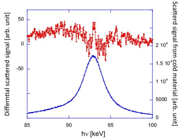
Fig. 4 Measured Compton spectrum (below) and the subtract result between that of cold material and that of laser heated expansion material. In the subtract data, the similar spectral response to the theoretical prediction is shown clearly.
