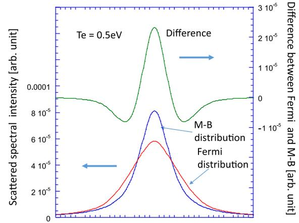
Fig. 2 Calculated spectrum of Compton scattering for two different electron velocity distribution function. The lower two spectrum denotes the spectrum of Fermi and M-B distribution. The upper curve is subtract results the lower two spectrums.
