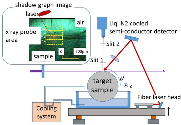
Fig. 3 Schematic drawing of inelastic Compton scattering measurement with CW high power laser. The inserted photograph is shadow graph picture for height level controller. The probe areas of  $>100$  keV x-ray are also shown in this picture.
