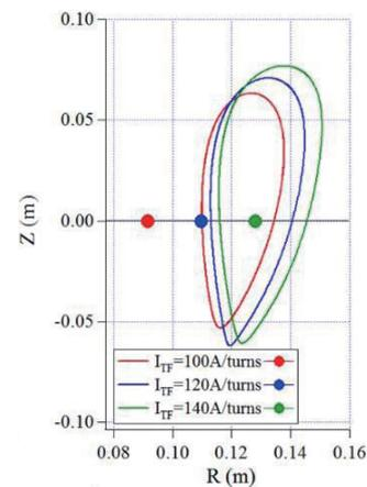
Fig. 6 The position of EC resonance layer (symbols) and the last closed magnetic surfaces calculated with HSD, for three values of the TF coil current. Red, blue and green symbols and curves denote the case with the TF coil current of 100 A, 120 A and 140 A, respectively.
