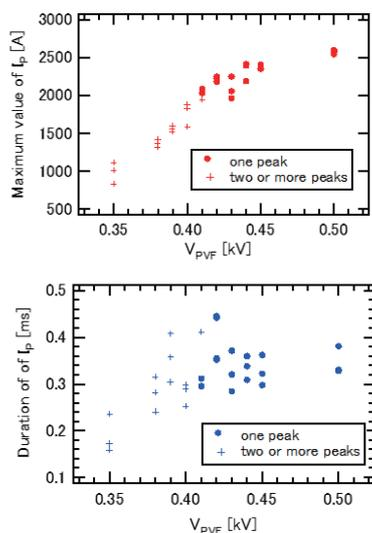
Fig. 5 (Top) The peak value of plasma current and (Bottom) the duration of plasma current as function of the charging voltage of the capacitor for the PVF coil circuit.
