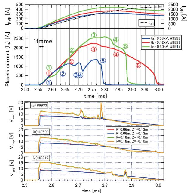
Fig. 3 Comparison of measured (Top) PVF coil current and plasma current waveform and (Bottom) loop voltages at  $R = 0.06$  m,  $Z = \pm 0.13$  m and  $R = 0.18$  m,  $Z = \pm 0.10$  m.
