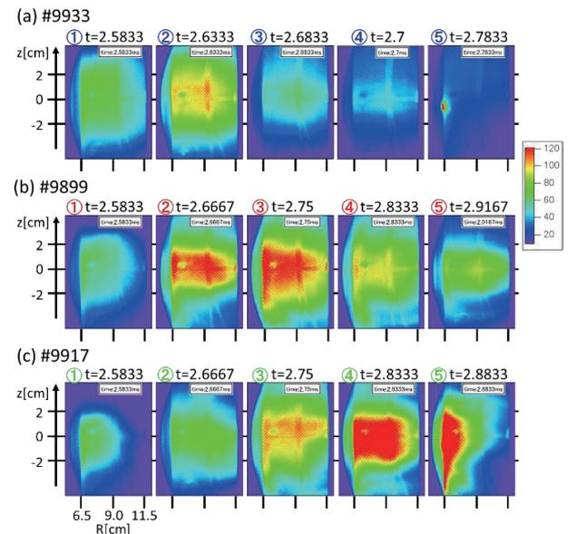
Fig. 4 Time evolution of images in tokamak discharge experiments for, (a)  $V_{PVF} = 0.38$  kV, (b)  $V_{PVF} = 0.42$  kV, and (c)  $V_{PVF} = 0.50$  kV.
