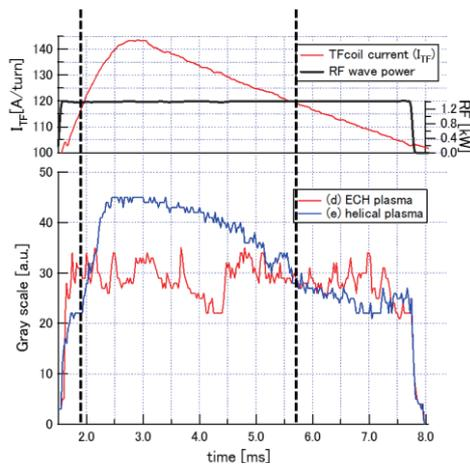
Fig. 8 (Top) Waveform of the TF coil current (in red) and the EC power (in black). (Bottom) Signals of light intensity of pixel at  $Z = -4$  cm without (in red) and with (in blue) helical field application.
