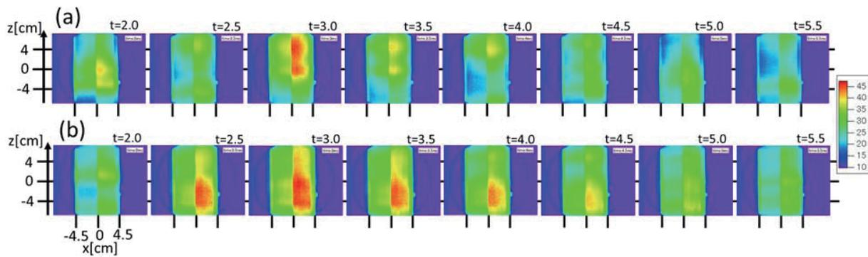
Fig. 7 Color images taken in the radial direction for (a) ECH plasma (TF+RF), (b) helical plasma (TF+RF+VF+HF+AHF).
