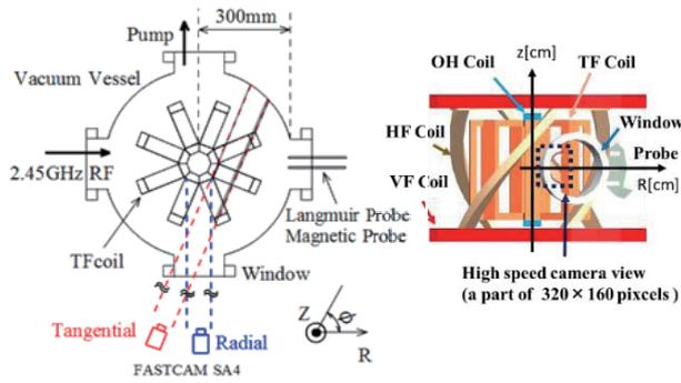
Fig. 2 (Left) Top view of high speed camera sightlines. (Right) Side view in the tangential direction.
