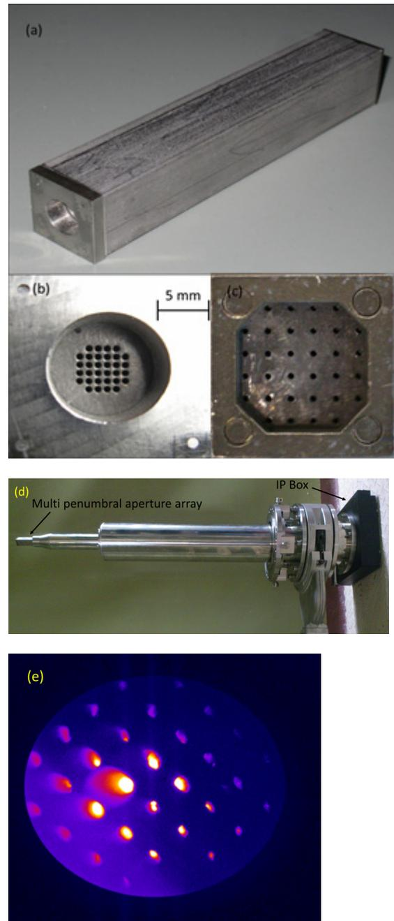
Fig. 7 (a) a picture of the multi penumbral aperture array, (b) front surface and (c) rear surface, (d) picture of the whole detector, (e) typical penumbral image obtained in the experiment.
