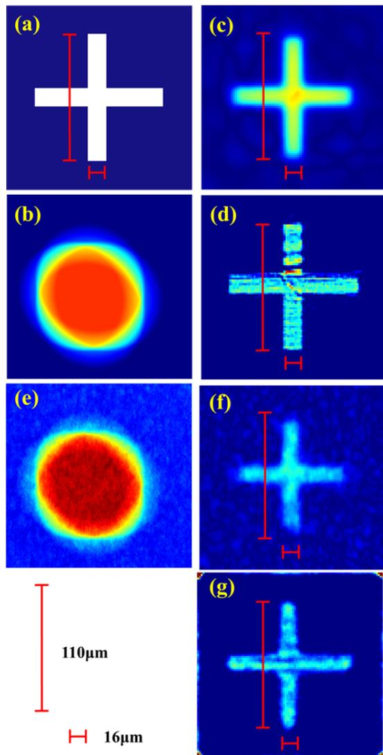
Fig. 2 Images obtained in the test reconstruction. (a) is cross pattern having  $110\mu\text{m}$  length and  $16\mu\text{m}$  width, (b) synthesized penumbral image, (c) reconstructed image using wiener filter based deconvolution, and (d) reconstructed image using newly developed method. (e) noise-added penumbral image, (f) reconstructed image from (e) by wiener filter based deconvolution, and (g) reconstructed image from (e) using newly developed method.
