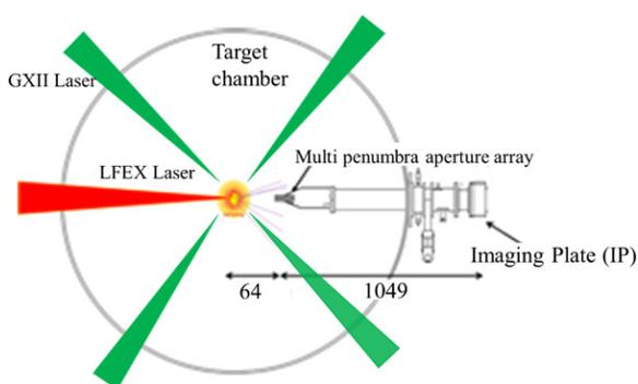
Fig. 6 Installation of multi penumbral diagnostic in the fast ignition experiment in the GEKKO XII and LFEX laser facility in Institute of Laser Engineering, Osaka University.
