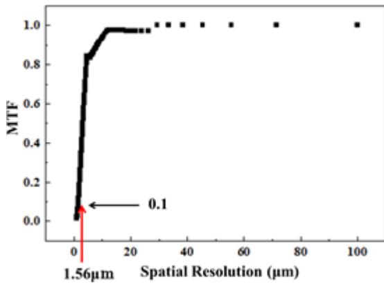
Fig. 4 Modulation transfer function curve obtained in a tested image by using newly developed Heuristic method.
