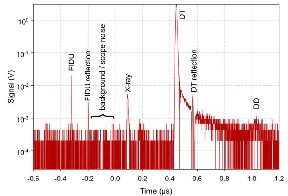
Fig. 2 Time-of-flight spectrum of the new nToF detector from an exploding pusher shot. Several features of the spectrum are visible: Fiducial signals for timing the X-rays from the shot as well as the DT neutron signal with a cable reflection.
