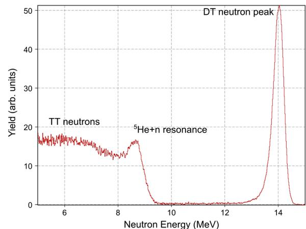
Fig. 3 TT neutron spectrum obtained from new nToF detector.
