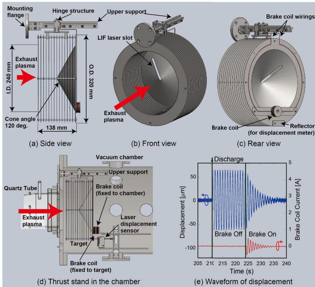
Fig. 2 Details of the thrust stand and waveform of the displacement.
