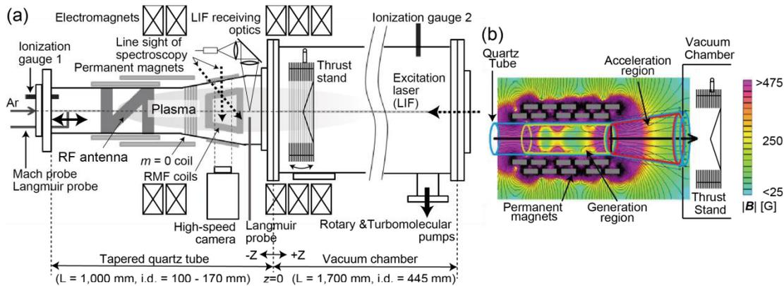
Fig. 1 Schematic of LMD and thrust stand (a) and magnetic field by permanent magnets (b).
