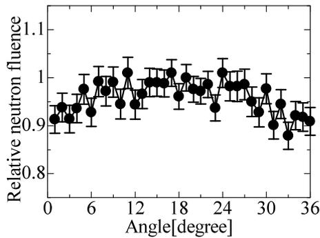
Fig. 8 Relative neutron fluence distribution with the supporting structures to without the structures.
