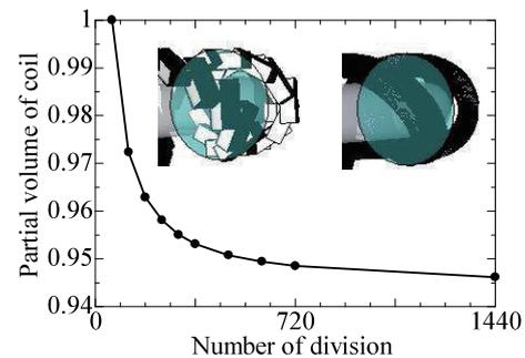
Fig. 4 Dependence of the partial coil volume between heights of the top and bottom ends of a plasma doughnut on the number of divisions. The ellipse of two pictures shows the area of coils we can see from an angle of 30 degrees for the O-port.
