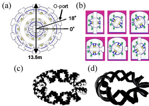
Fig. 1 Schematic view of the geometry used in MCNP code. (a) Horizontal section on the equatorial plane of LHD. (b) Vertical sections at different angle positions. (c) Coils divided into 60 areas. (d) Coils divided into 1440. When number of divisions increases, the shape of coils can be smooth from a square shape segmented coil to a seamless coil.
