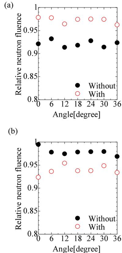
Fig. 6 Neutron fluence distribution. (a): above the supporting structures. (b): below the supporting structures. Fluences with and without the structures are plotted. Statistic uncertainty is less than 1%.
