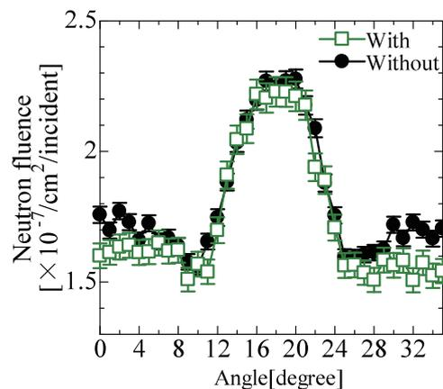
Fig. 7 Neutron fluence distribution outside the O-port. Open squares and closed circles show the neutron fluences with and without the supporting structures, respectively. Statistic uncertainty is less than 5%.
