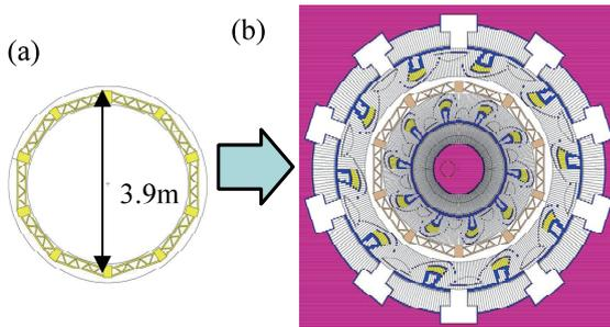
Fig. 5 (a) Schematic top view of the geometry of supporting structures. A large circle indicates the area of the vacuum vessel. (b) Horizontal section with supporting structures, which colored pink, at the 50 cm low position from the equatorial plane of LHD.
