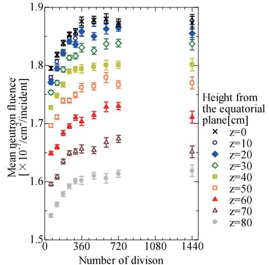
Fig. 3 Mean neutron fluences in the region of toroidal angles from 15 to 21 degrees. Results at various heights from the equatorial plane are plotted. Error bars show statistical uncertainty.
