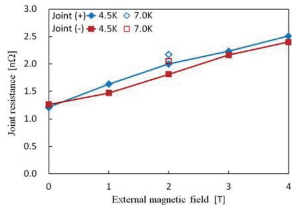
Fig. 4 Joint resistance of the joint samples.
