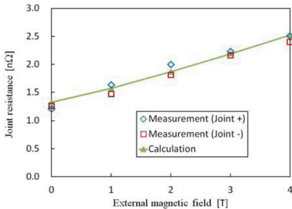
Fig. 6 Comparison between measurement and calculation with regard to joint resistance at 4.5 K.
