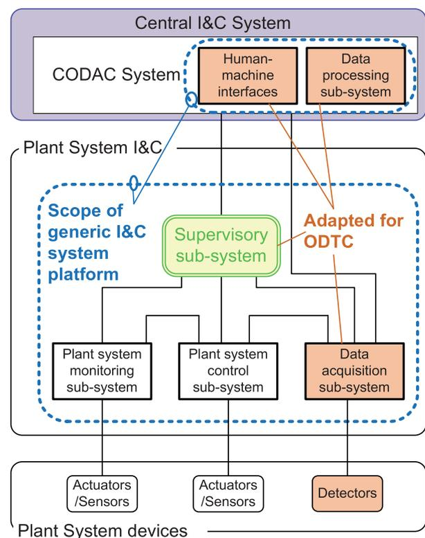
Fig. 3 Overview of the designed generic I&C system platform and sub-systems adapted for ODTC system.
