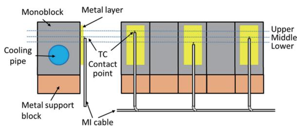
Fig. 2 Cross-section and side view of ODTC components mounted on divertor monoblocks. They are heated on the plasma facing top, and cooled by water through the cooling pipe.
