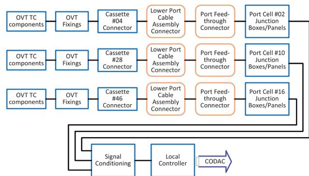
Fig. 1 System Overview of the ODTC system. There are 3 sets of TC components and cabling for 3 divertor targets, and one I&C system.
