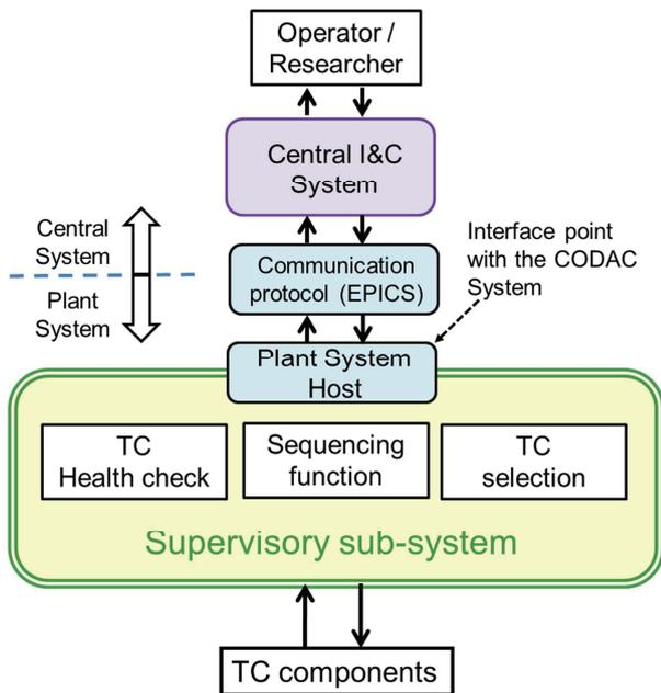
Fig. 4 Schematic view of the supervisory sub-system for the ODTc system.
