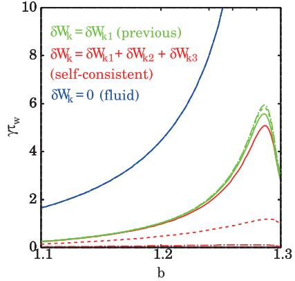
Fig. 2 RWM growth rates normalized by the inverse of the wall diffusion time as functions of wall location.
