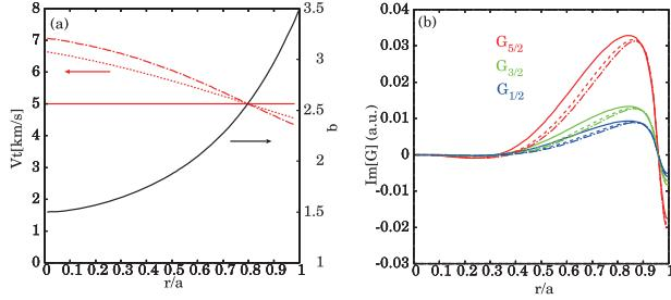
Fig. 1 (a) A fixed safety factor profile (black) and various rotation profiles (red). (b) Radial profiles of  $G$  factors for various rotation profiles.
