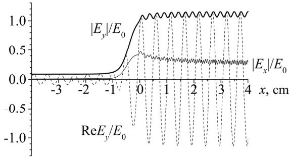
Fig. 3 Calculated profiles of  $|E_y|$  (heavy solid line) and  $|E_x|$  (light solid line) near the resonance  $\omega_0 = 2\omega_{ce}$ . The dashed line shows  $\text{Re}E_y$  as a function of  $x$  at a certain instant of time. The fields are normalized to the amplitude  $E_0$  of the incident wave in vacuum.
