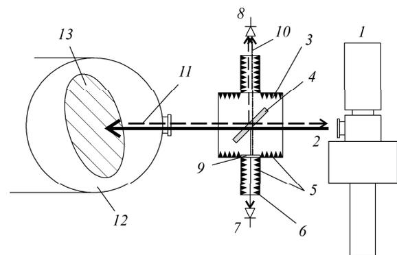
Fig. 1 Scheme of the experiment on the detection of backscattered gyrotron radiation in the L-2M stellarator: (1) gyrotron, (2) gyrotron radiation, (3) quasi-optical coupler, (4) mica splitter, (5) absorber, (6) radiation collimator, (7) detector of the gyrotron radiation power, (8) detector of scattered radiation, (9) polarization grid, (10) reference beam, (11) backscattered radiation, (12) cross section of the vacuum chamber, and (13) cross section of the plasma column.
