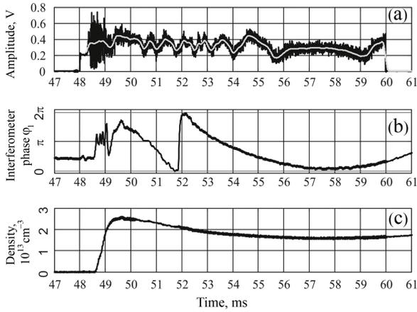
Fig. 2 (a) Signal of the homodyne detector before and after averaging over the time interval of  $300\ \mu\text{s}$  (1500 readings) and the time dependences of (b) the phase increment of the interferometer measuring the plasma density along the central horizontal chord and (c) the average plasma density.
