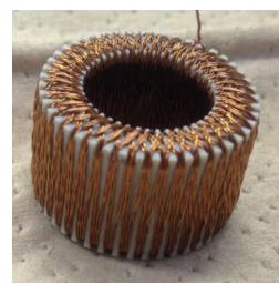
Fig. 4 Eight-layer Rogowsky coil: Outer diameter = 20 mm; inner diameter = 12 mm; thickness = 12 mm; number of turn 360; sensitivity =  $5.0 \times 10^{-7}$  Vs/A; and thickness of the cable = 0.12 mm.
