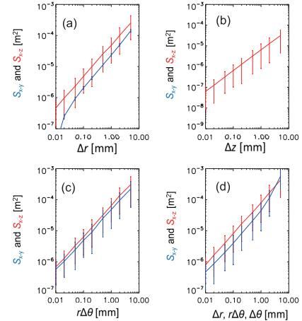
Fig. 2  $S_{x-y}$  and  $S_{x-z}$  of the two layer winding, where,  $\Delta r$ ,  $\Delta z$  and  $r\Delta\theta$  are errors in each direction.
