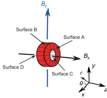
Fig. 1 A Rogowski coil in a tokamak discharge.
