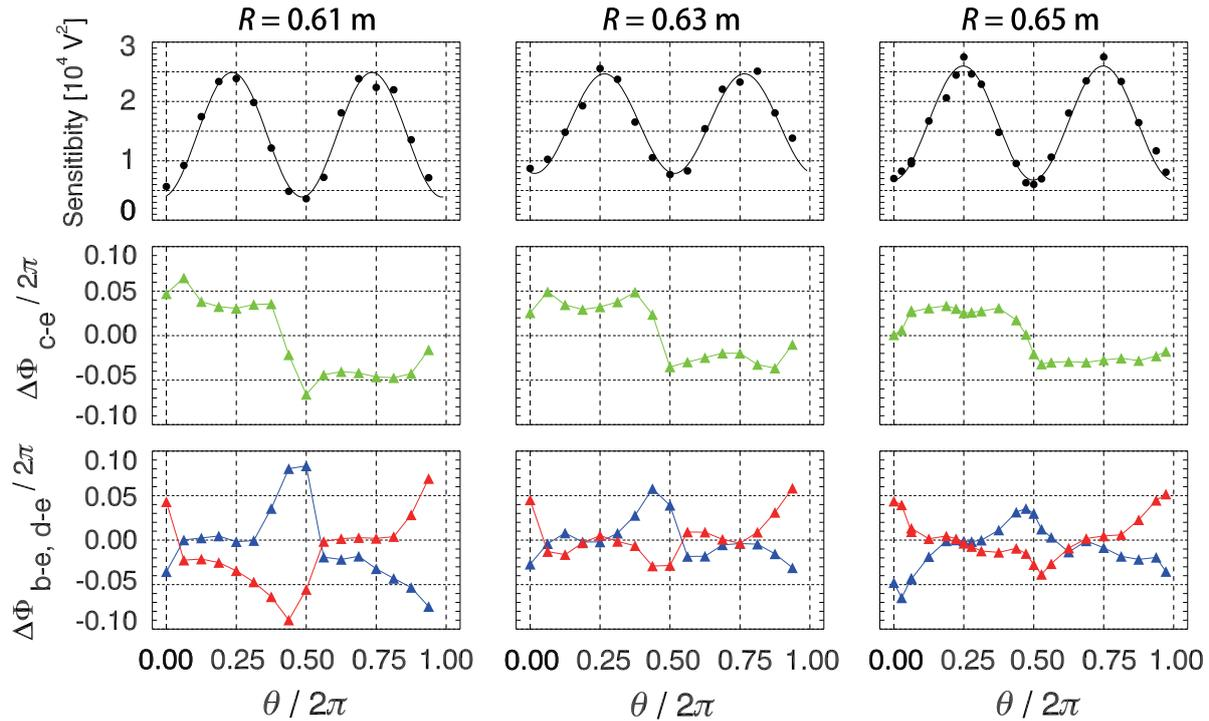
Fig. 4 Squared voltage (top) and phase differences between e and other channels (2nd and 3rd rows) at 200 MHz plotted as functions of the normalized angle  $\theta/2\pi$ . The green, blue, and red symbols represent  $\Delta\phi_{c-e}$ ,  $\Delta\phi_{b-e}$ , and  $\Delta\phi_{d-e}$ , respectively.
