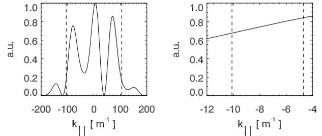
Fig. 3 The parallel wavenumber ( $k_{\parallel}$ ) spectrum in front of the grill antenna. The 5ch-RFMP can detect  $|k_{\parallel}| < 105$   $\text{m}^{-1}$ . The figure on the right shows the  $k_{\parallel}$  spectrum on an expanded scale.
