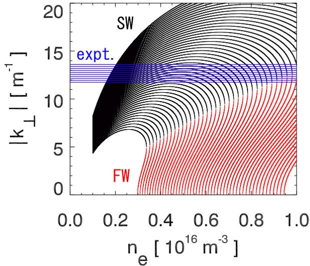
Fig. 5 The cold plasma dispersion relation. Black lines represent the SW. Red lines represent the FW.  $|k_{\perp}|$  is calculated from the dispersion relation using the measured  $k_{\parallel}$  at  $R = 0.63$  m,  $B_t = 0.04$  T, and  $n_e$  in the range  $10^{15-16} \text{ m}^{-3}$ . The blue lines mark the range of measured  $|k_{\perp}|$  at  $R = 0.63$  m.
