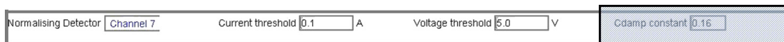
Fig. B4c AELM normalization channel selection, in this shot channel-7 = I_{ANT7} (out of the 22 possible engineering signals connected to the AELM) was selected for the AGC current control algorithm and used to normalize the measured signal for the AELM real-time mode detection and tracking algorithm (parameters not relevant for this choice of normalization channels have been shaded in this figure).
