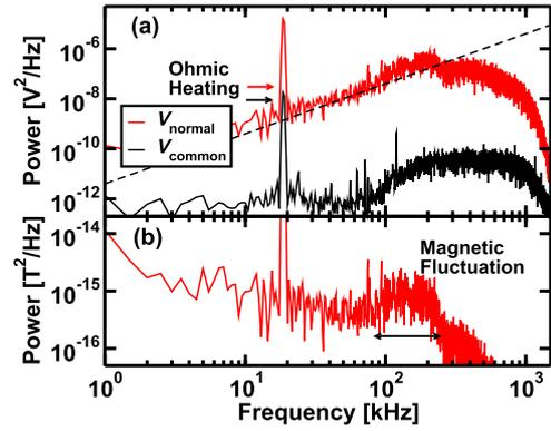
Fig. 4 (a) The power spectra of normal mode signal  $V_{\text{normal}}$  and common mode signal  $V_{\text{common}}$  at  $\rho \sim 0.2$  and a square of frequency (dash line) and (b) the power spectra of magnetic field fluctuation.
