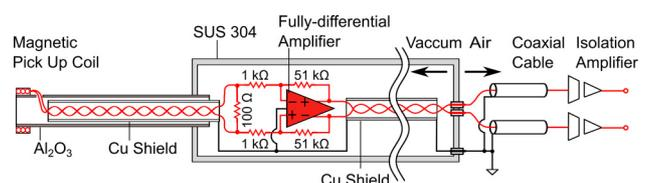
Fig. 1 Schematic of magnetic probe.
