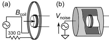
Fig. 2 (a) Schematic of the magnetic sensitivity calibration and (b) CMRR measurement.
