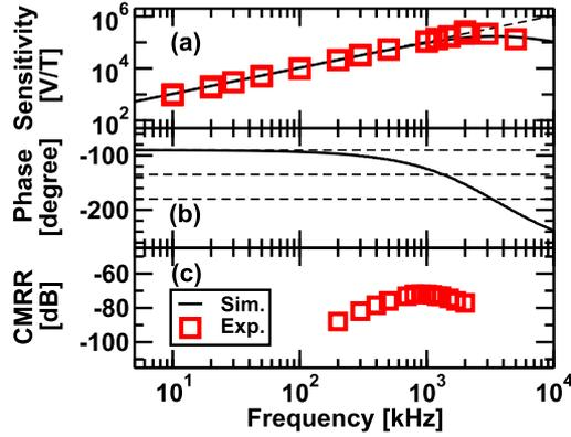
Fig. 3 (a) The frequency dependence of the magnetic sensitivity, (b) phase difference between magnetic field  $B_{\text{coil}}$  and normal mode signal  $V_{\text{normal}}$ , and (c) CMRR measurements.
