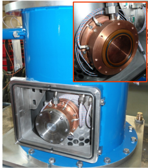
Fig. 8 Picture of the cryogenic prototype laser head to be operated with a 77 mm diameter \text{Yb}^{3+}/\text{Cr}^{4+} :YAG gain medium. The top right insert displays the copper side of the Helium cell.
