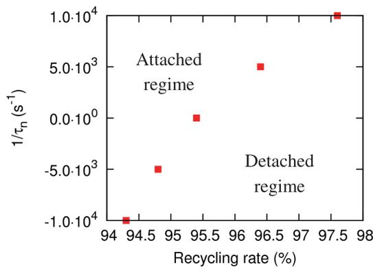
Fig. 5 Conditions of recycling rate and cross-field neutral loss time constant for detached regime to occur.
