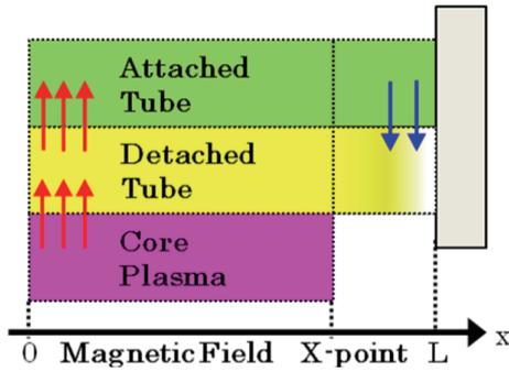
Fig. 1 Schematic picture of (multi-layer) 1D divertor model.
