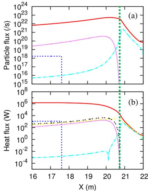
Fig. 4 Spatial (a) particle and (b) heat flux profile. Red lines represent local particle and heat flux. Blue input from the core plasma, pink ionization, aqua (absolute) recombination, yellow charge exchange, black impurity radiation. Detachment front is denoted by the vertical broken green line.
