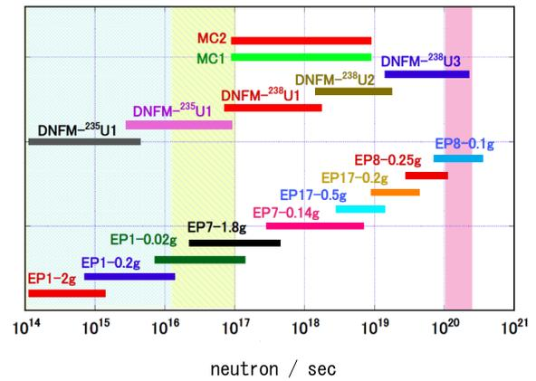
Fig. 1 Dynamic ranges covered by neutron flux monitors in counting mode, with time-resolution of 1 ms. With time resolution of 10 ms, ranges extend to the regions of one-order lower. The left shadowed area (blue) shows that is attainable in calibration experiments with a generator of  $10^{10}$  n/s in  $10^4$  sec. The right shadowed area (pink) shows the region of the high performance DT operation.
