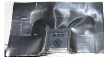
Fig. 3 External appearance of an OPERA film used in the NSTX. The emulsion is vacuum-packed using a thin aluminum sheet.
