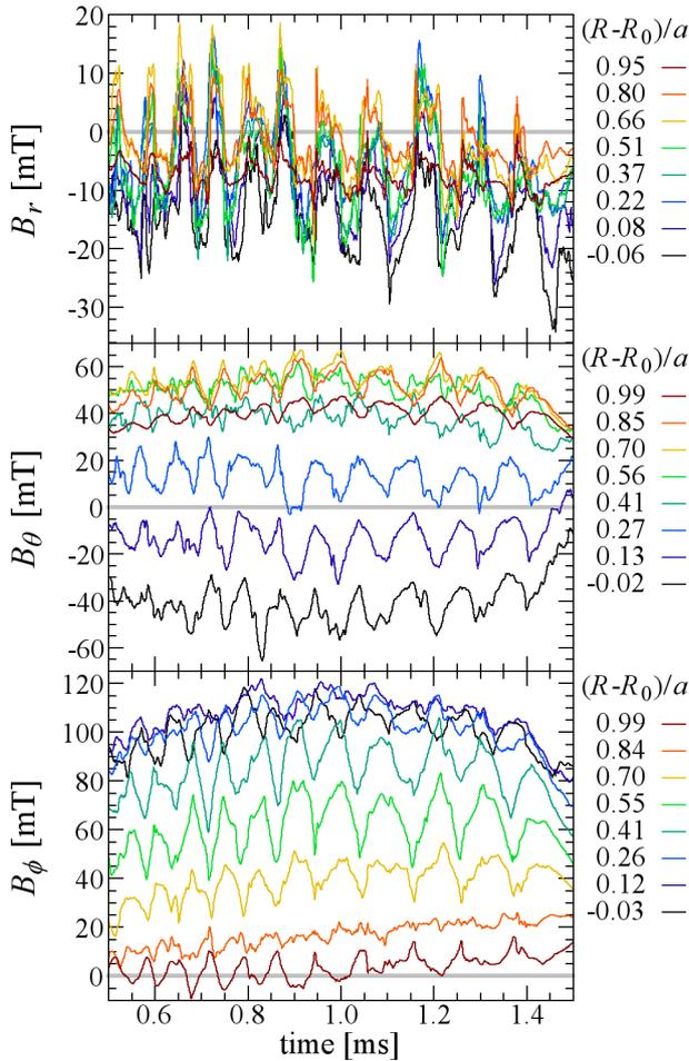
Fig. 4 Time evolution of magnetic fields measured by the radial array.
