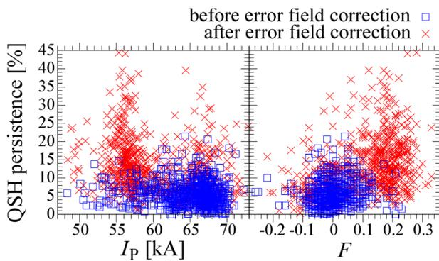
Fig. 7 QSH fraction (persistence) in the flat-topped current phase vs. plasma current  $I_p$  and  $F$  before and after the error field correction by the poloidal flange modification. The data set consists of results from more than 1000 shots.
