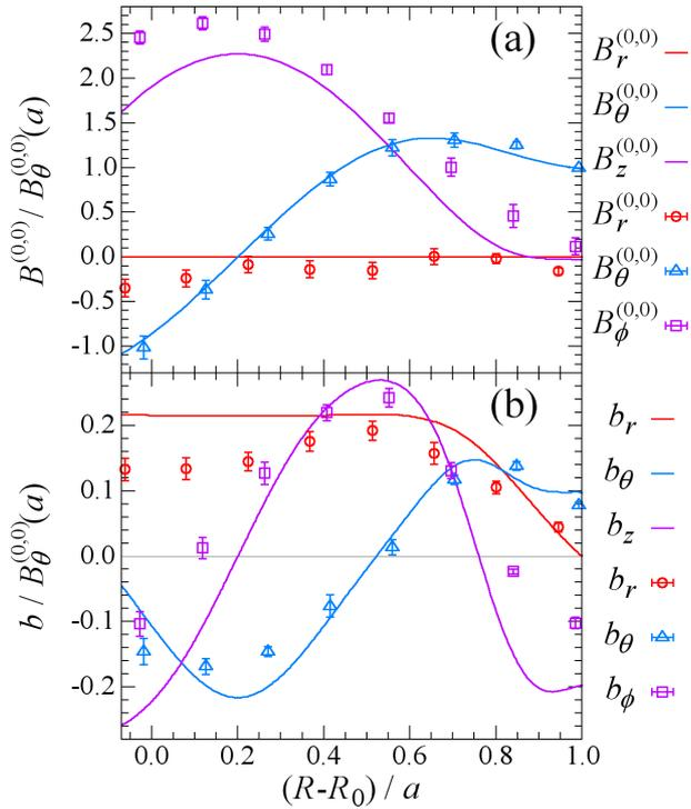
Fig. 6 Comparison of radial profiles of magnetic fields of experiment (dots) and the theoretical helical Ohmic equilibrium (lines). (a) is the experimental non-oscillating ( $< 2$  kHz) component averaged over the flat-topped phase in 5 discharges and the theoretical poloidally and toroidally symmetric component. (b) is the experimental time averaged amplitude of oscillating (2-50 kHz) component averaged over the 5 discharges and the theoretical helical component.
