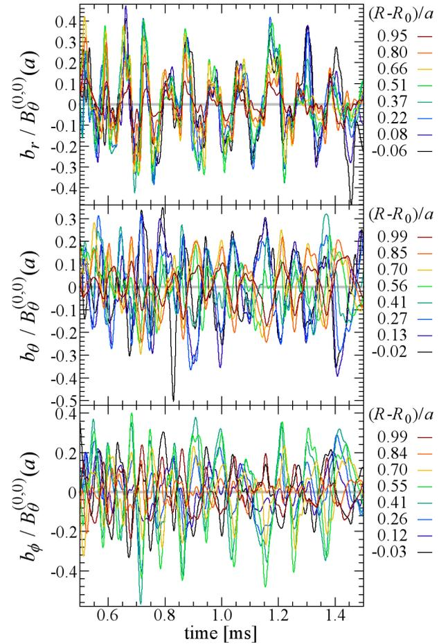
Fig. 5 Time evolution of oscillating (2-50 kHz) component  $b$  of magnetic fields measured by the radial array, which is normalized by the non-oscillating (< 2 kHz) component of an edge poloidal magnetic field  $B_\theta^{(0,0)}(a)$ .
