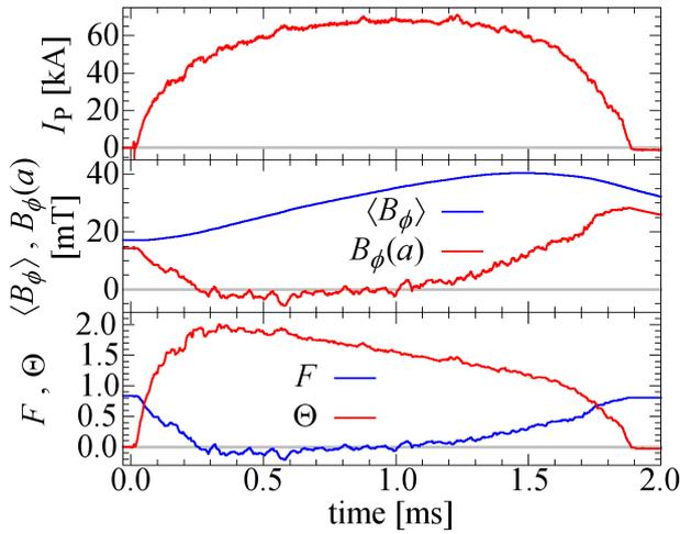
Fig. 2 Time evolution of the plasma current  $I_p$ , average toroidal magnetic field  $\langle B_\phi \rangle$ , averaged edge toroidal magnetic field  $B_\phi(a)$ , field reversal parameter  $F$ , and pinch parameter  $\Theta$  in a typical QSH discharge in RELAX.
