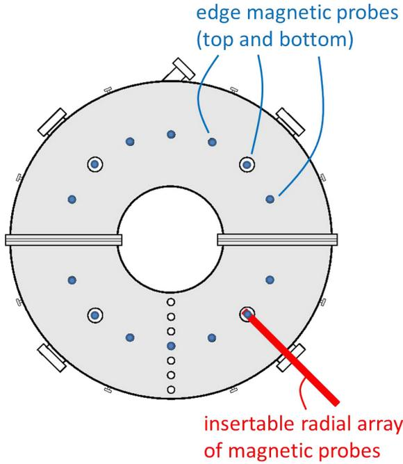
Fig. 1 Top view of RELAX with arrangement of magnetic diagnostics.
