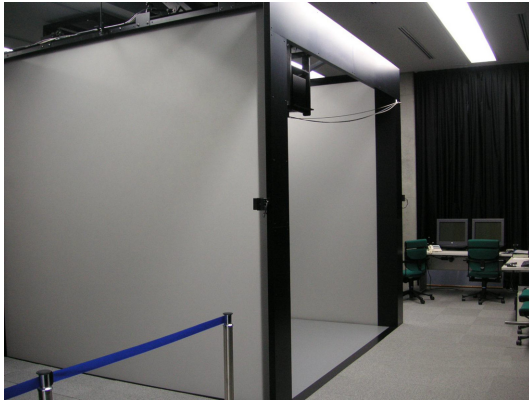
Fig. 1 CAVE system at Earth Simulator Center, JAMSTEC. The size of screens is 3\text{ m} \times 3\text{ m} each.
