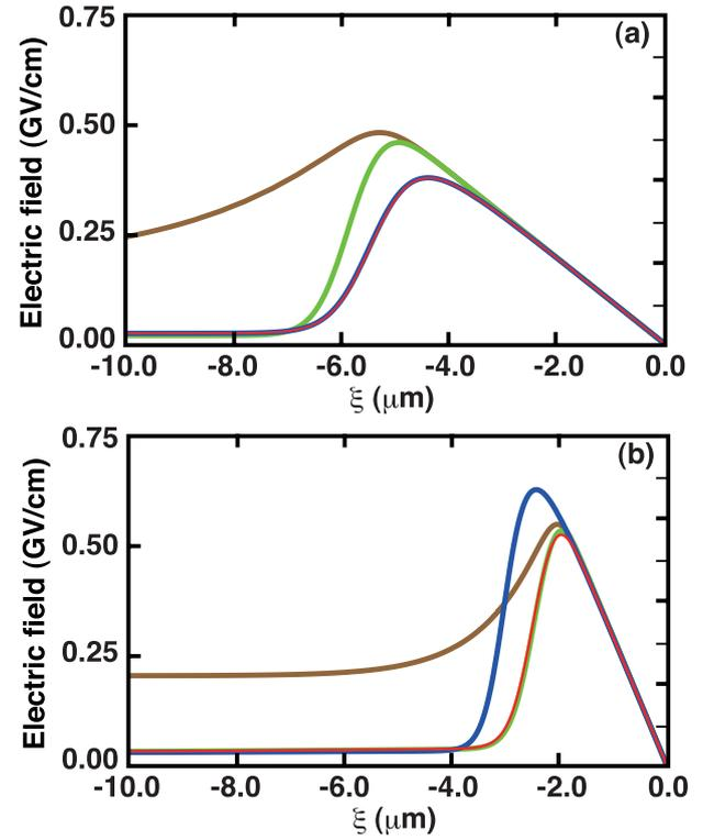
Fig. 2 Electrostatic field profiles for (a)  $n_b/N = 1 \times 10^{-5}$  and (b)  $n_b/N = 3 \times 10^{-5}$ , respectively. The colors of the lines represent the same features outlined in Fig. 1.
