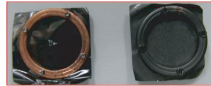
Fig. 1 The foil mounted in copper gasket. Left foil is single sided blackened foil. Right foil is double sided blackened foil.
