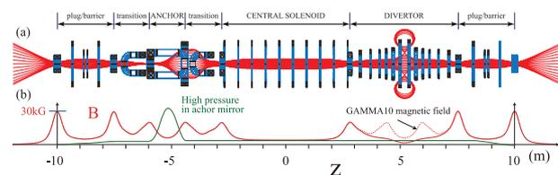
Fig. 1 GAMMA10 A-divertor. (a) is the magnetic field lines with coils and (b) is the axial magnetic field and pressure profiles.
